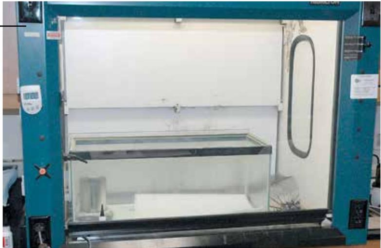
**FIGURA 11-5***Cámara de deposición de metal al vacío.*
