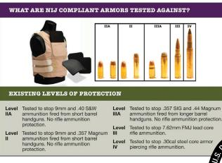
There are currently five different body armor performance levels, which are based on the vests' protection against various kinds of ammunition. Regardless of performance level, NIJ requires the vests to protect against both perforation and blunt trauma.27
