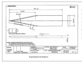
This engineered knife blade, which is typical of small knives, was used to help fashion the stab/slash performance standards. With a pointed tip and stiff backbone, it is thinner than other blades and has just one cutting edge.<sup>31</sup>
