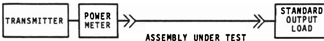
FIGURE 2. Block diagram for SWR measurement.
