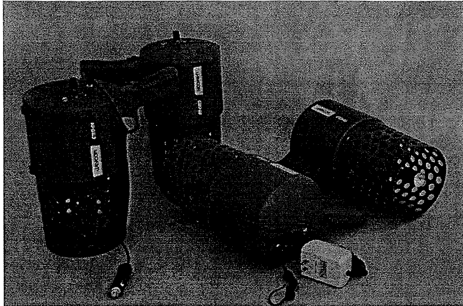
Figure 5. Later working models of the handheld ultrasound concealed-weapons detector.
