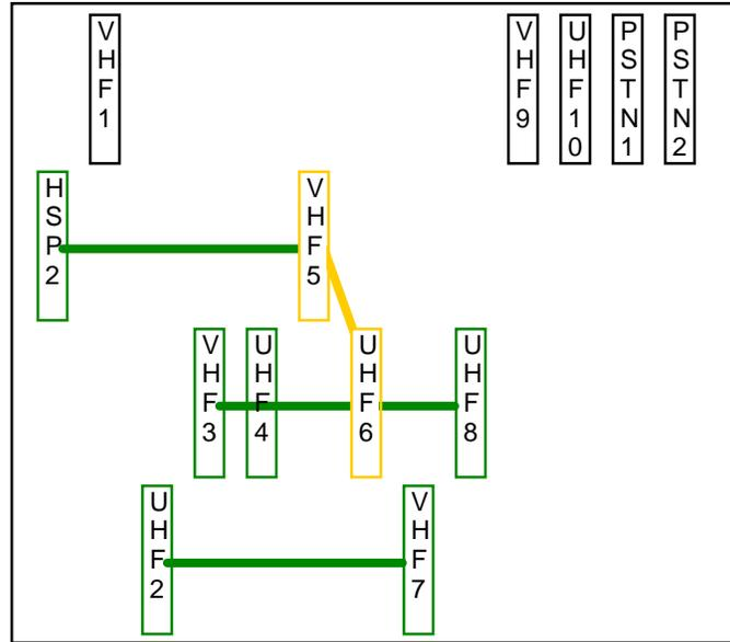
Figure 7. Example network configuration with two interconnected nets.
