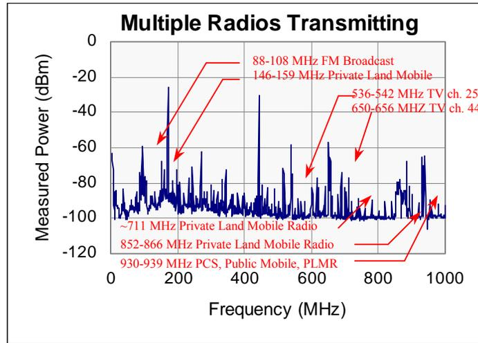
Figure 17. Seven radios simultaneously transmitting into dummy loads.
