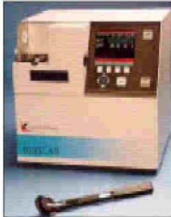
**Figure 3.1.1.1-1 Front view of IONSCAN 400B with swab sampler.**
