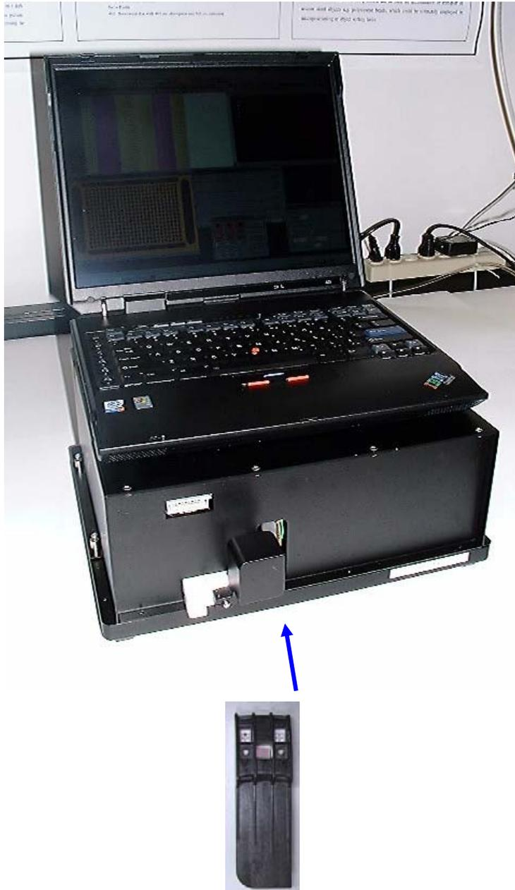
**Figure 17. Nanogen's portable electronic microarray system with the laptop used to operate the instrument and perform data storage and processing. A port for the 400-site cartridge is labeled separately (not to scale with the instrument).**
