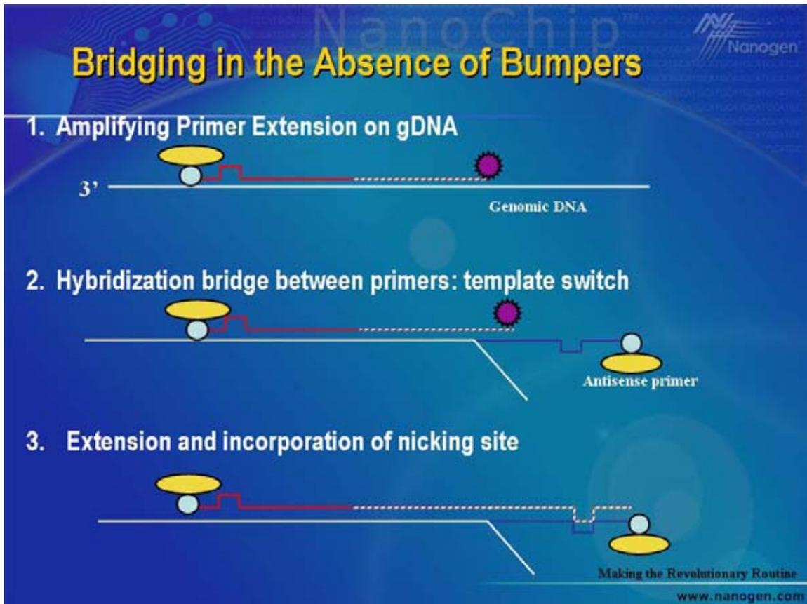
Figure 6a – 1) Genomic DNA hybridizes to a primer and is extended by the polymerase. 2) The end of the extended duplex “breathes”. This partial dehybridization permits an antisense primer in close proximity to hybridize and provide a template for the polymerase. 3) The polymerase can now use the antisense primer as a template and incorporate the nicking site.
