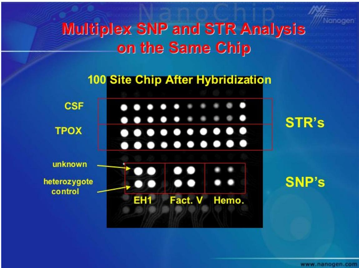
**Figure 9 – Multiplex SNP and STR Analysis on the Same chip a) – Image of fluorescence detected as a result of hybridization of targets and probes.**
