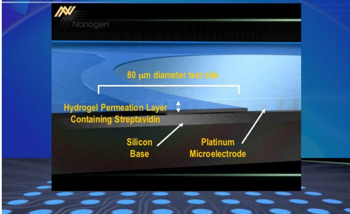
Figure 18 – Cartoon of the cross section of an electronic pad showing the distribution of the permeation layer
