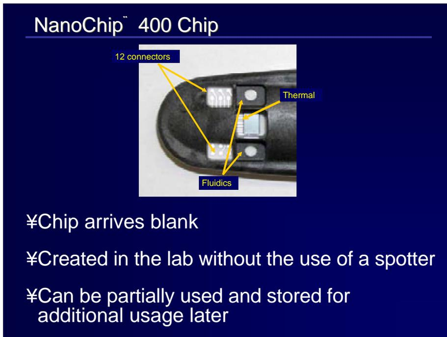
**Figure 14b – A view of the “hard” instrument interfaces of the chip. Note that the on-board switching permits control through only 12 connectors. The optical window is on the opposite side.**
