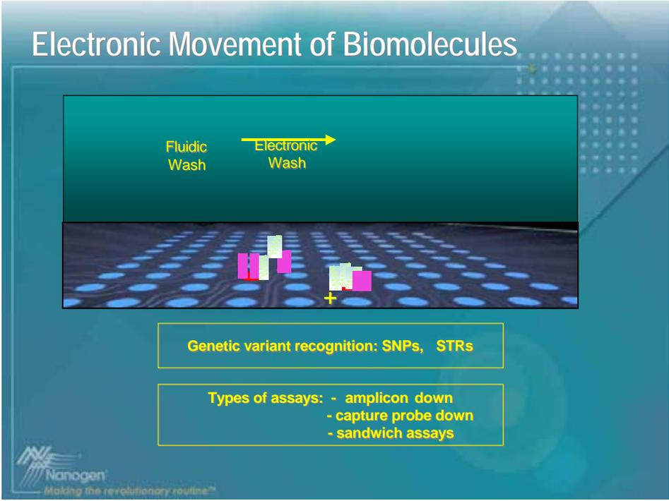
**Figure 2d – Electric field concentration of charged molecules drives an attachment reaction between moieties on the mobile molecules (biotin) and complementary entities imbedded in the permeation layer (streptavidin)**
