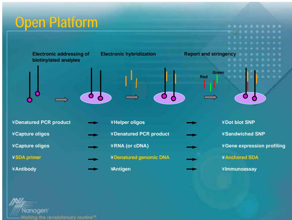
**Figure 1 – Examples of different electronic Microarray assay formats.**
