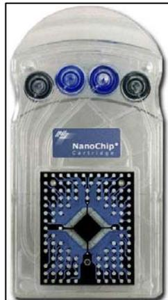
**Figure 13. The NanoChip® 100-site electronic microarray is contained within a plastic cartridge with fluidic ports.**
