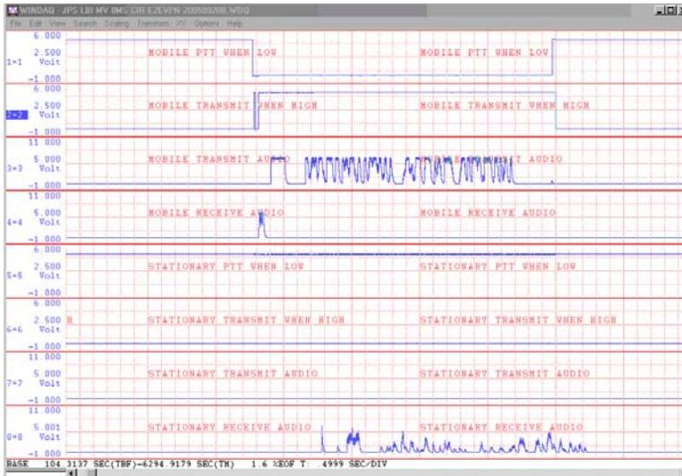
Figure 11 TYPICAL SAT TERMINAL ORIGINATED CALL.GIF
