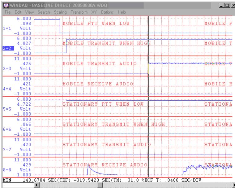
Figure 4 DIRECT PREAMBLE TX START.GIF
