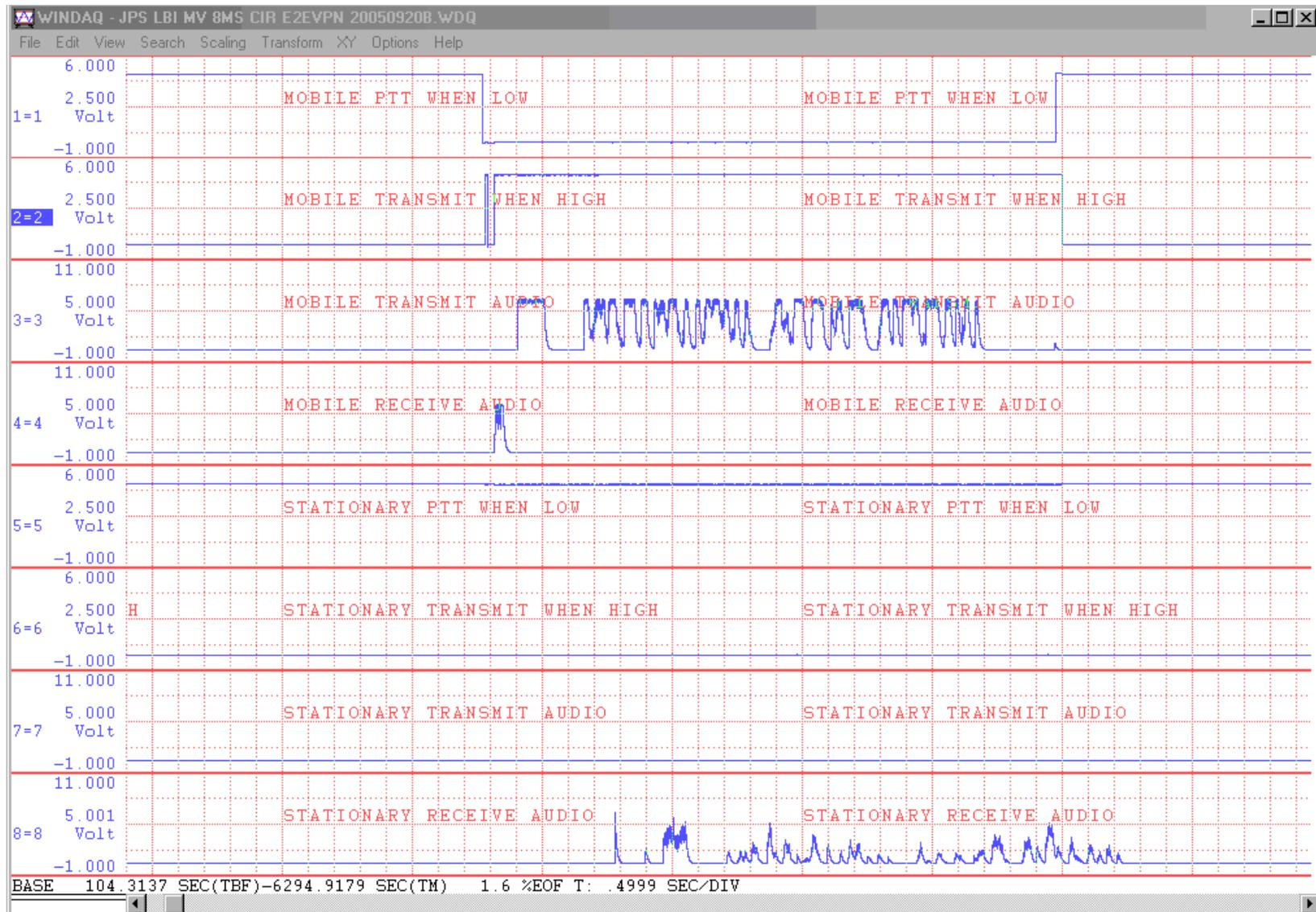
FIGURE 11 TYPICAL SAT TERMINAL ORIGINATED CALL.GIF
