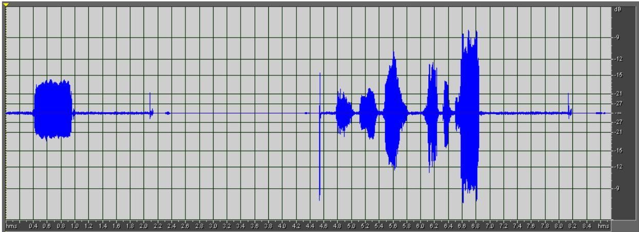
Figure 16 TYPICAL INTERFERENCE LIMITED AUDIO.GIF
