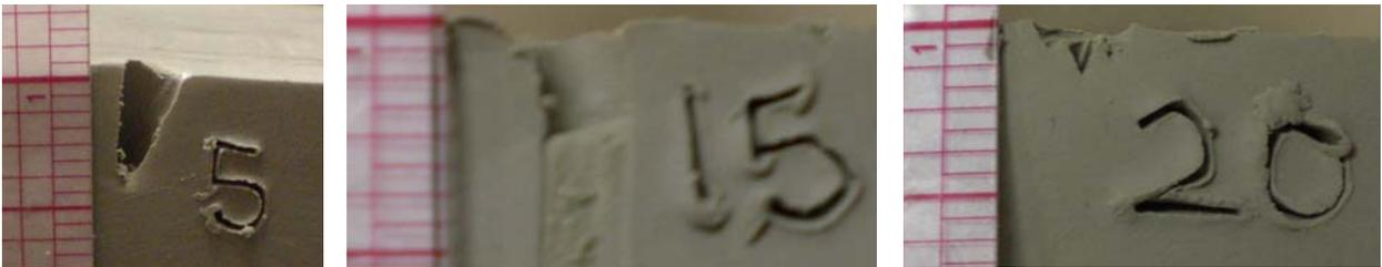
At the 10-foot distance interval the TASER barb penetrated fully and the base of the probe also penetrated the ballistic clay to about the same depth as probe base at the 5-foot distance interval.
