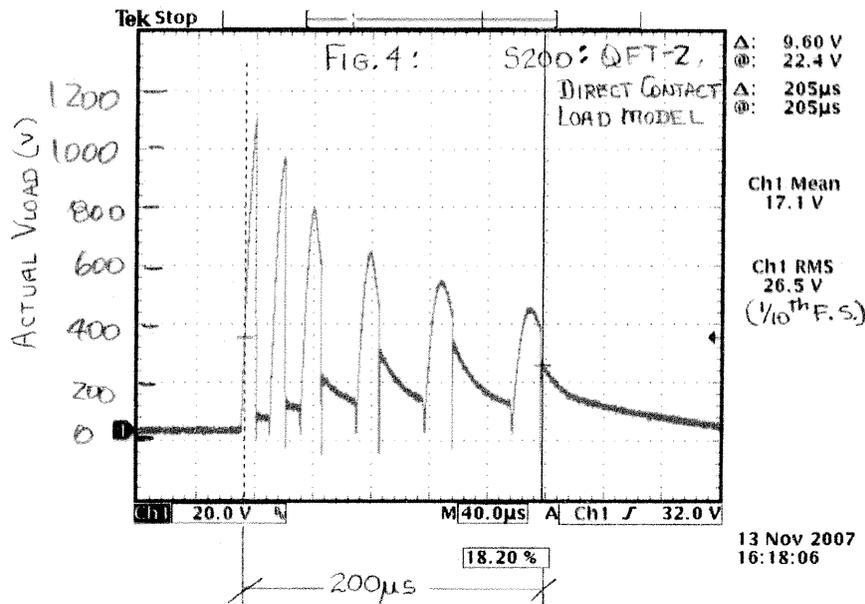
**Figure 5:** The S-200 Output Voltage Waveform: Clothed Target Load
