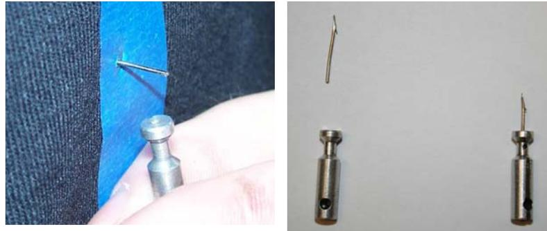
In addition to capturing images of this, the researchers developed a variable “Did Probe Break” which was used to capture whether the base of the probes separated from the barb which was fixed in the target. Of concern here is whether or not an officer would be able to process a subject into a correctional facility if they required the medical or surgical removal of a barb.
