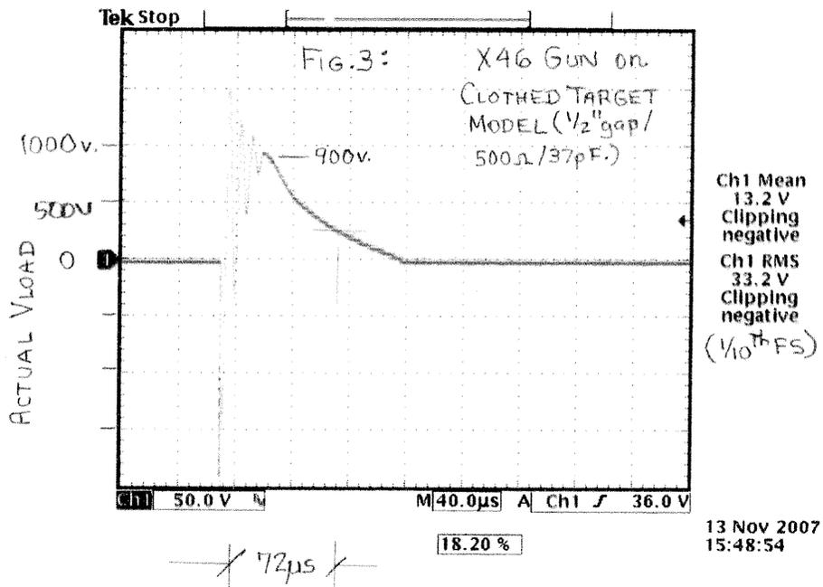
**Figure 4:** The S-200's Output Voltage Waveform: Direct Contact
