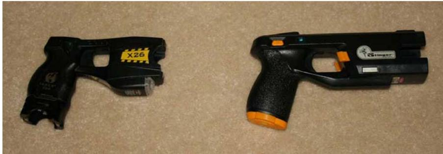
On the Stinger S200, the cartridge fits inside the weapon and is removed with an ambidextrous magazine release near the front of the gun. This spring-loaded action forces the cartridge out of the gun. The on/off switch on the Stinger S200 is a cross bolt design (similar to the Remington 870 shotgun safety-switch) and is located above the grip, on the frame of the weapon.
