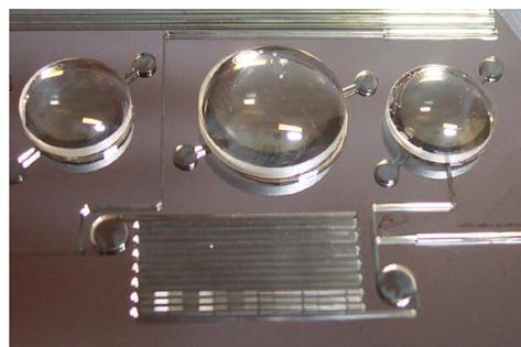
**Figure 10. EHP pumps integrated into a complete testing system.** Small disks next to lenses are fill pads while larger pads next to microfluidic channels are bubble traps.
