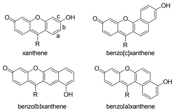
**Figure 1.** The xanthene dye framework (upper left, typified by fluorescein) and three types of benzoxanthenes. Benzoxanthene types are each distinguished via the orientation of their naphthyl moieties. We have synthesized the first known benzo[b] and [c]xanthenes and have prepared the benzofluorones corresponding to types a, b, and c. The benzofluorones, unlike xanthenes such as fluorescein, do not contain carboxylic acid/lactone moieties and thus are not quenched below pH = 5 (see Figure 2).
