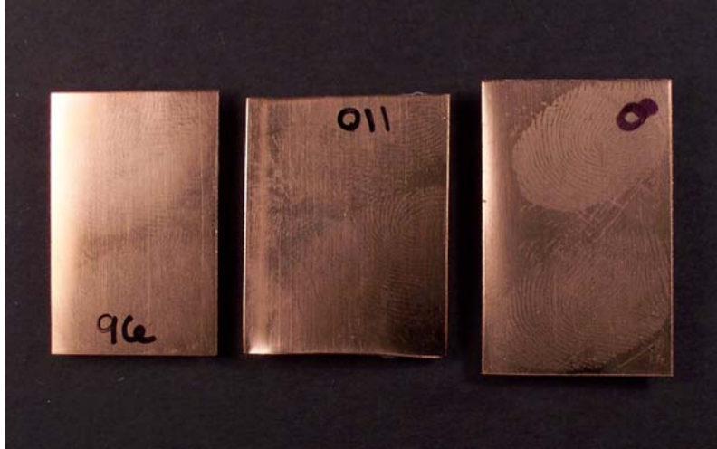
Copper sheet temperatures from left to right; 69° F, 71° F, 68° F, simultaneously processed with cyanoacrylate fuming showing effects of temperature variable on deposition.
