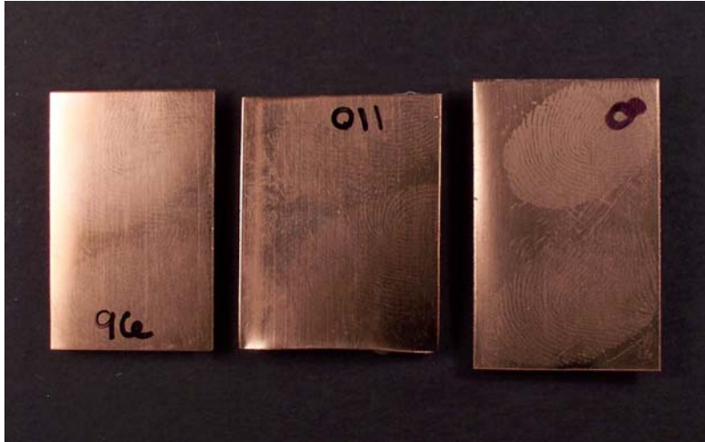
Copper sheet temperatures from left to right; 69° F, 71° F, 68° F, simultaneously processed with cyanoacrylate fuming showing effects of temperature.
