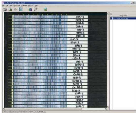
1. Batches of up to forty-eight strips are assembled on a custom holding plate, and digitally imaged using a common flatbed scanner
