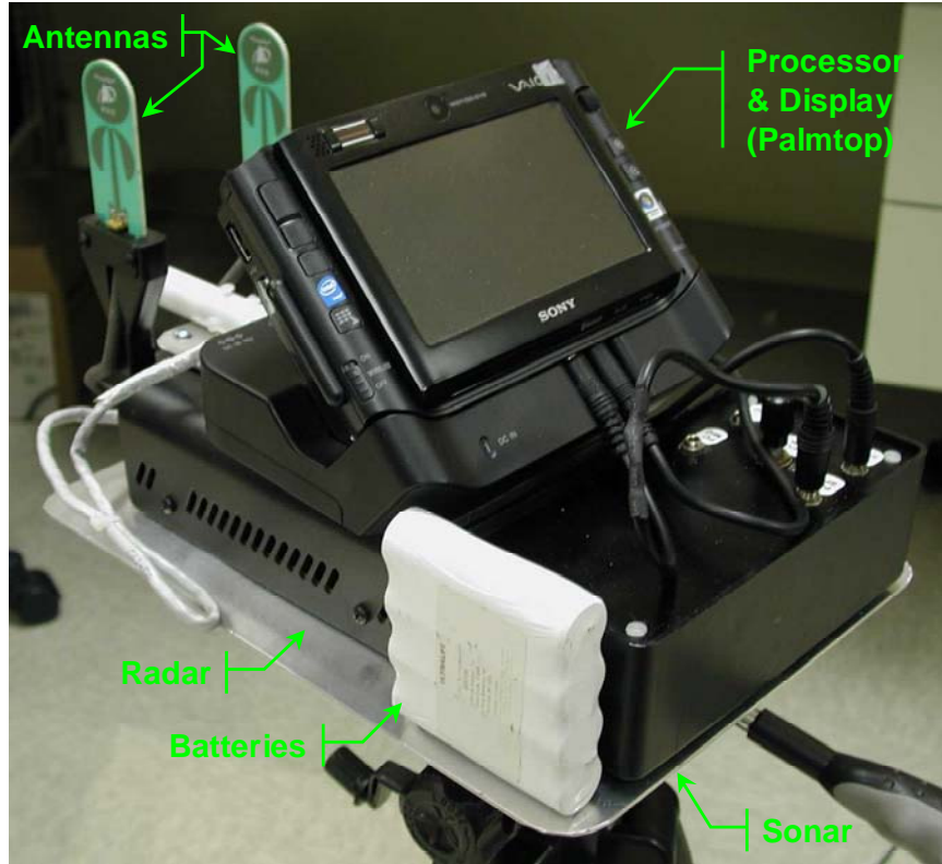
Figure 8: Photograph of Back of Assembled Unit, Sonar and Radar.
