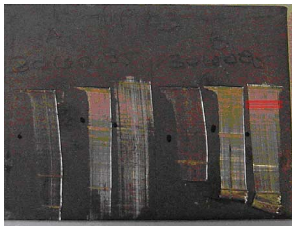
Figure 6. Marked lead sample with red lines representing profilometer traces.
