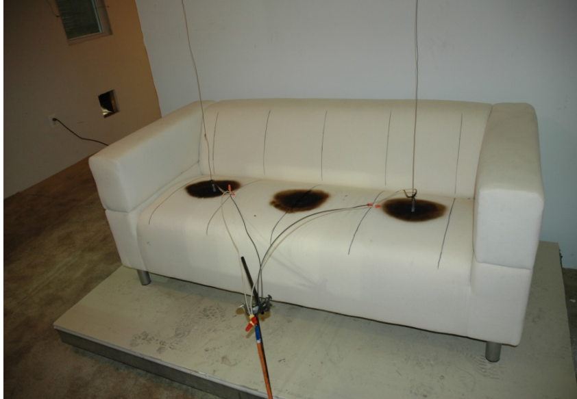
Figure 5-16. Test SM3 damage (the center char area is from test SM2)
