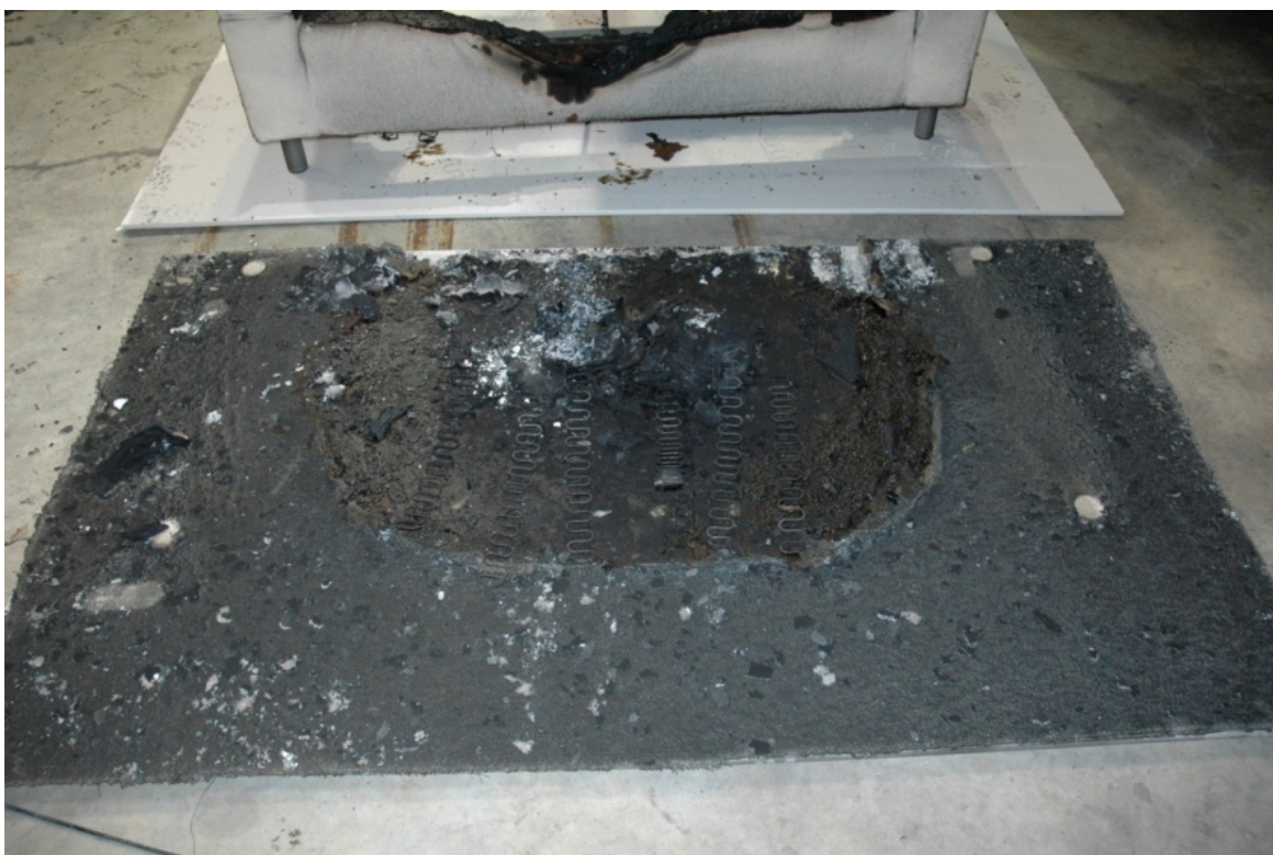
Figure 8-6. Burn pattern under sofa common to all accidental tests.
