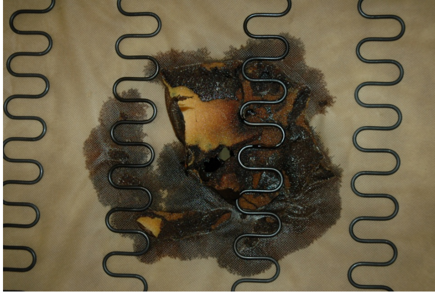
Figure 5-18. Close-up view of damage to underside of sofa seat caused in SM2, SM3
