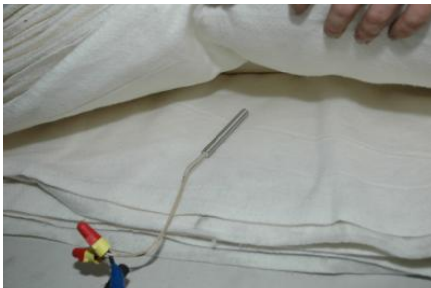
Figure 5-12. Cartridge heater position during test SM1
