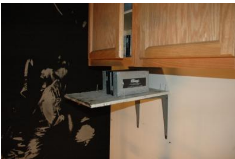
Figure 5-40. Ignition scenario for high cabinet flaming tests
