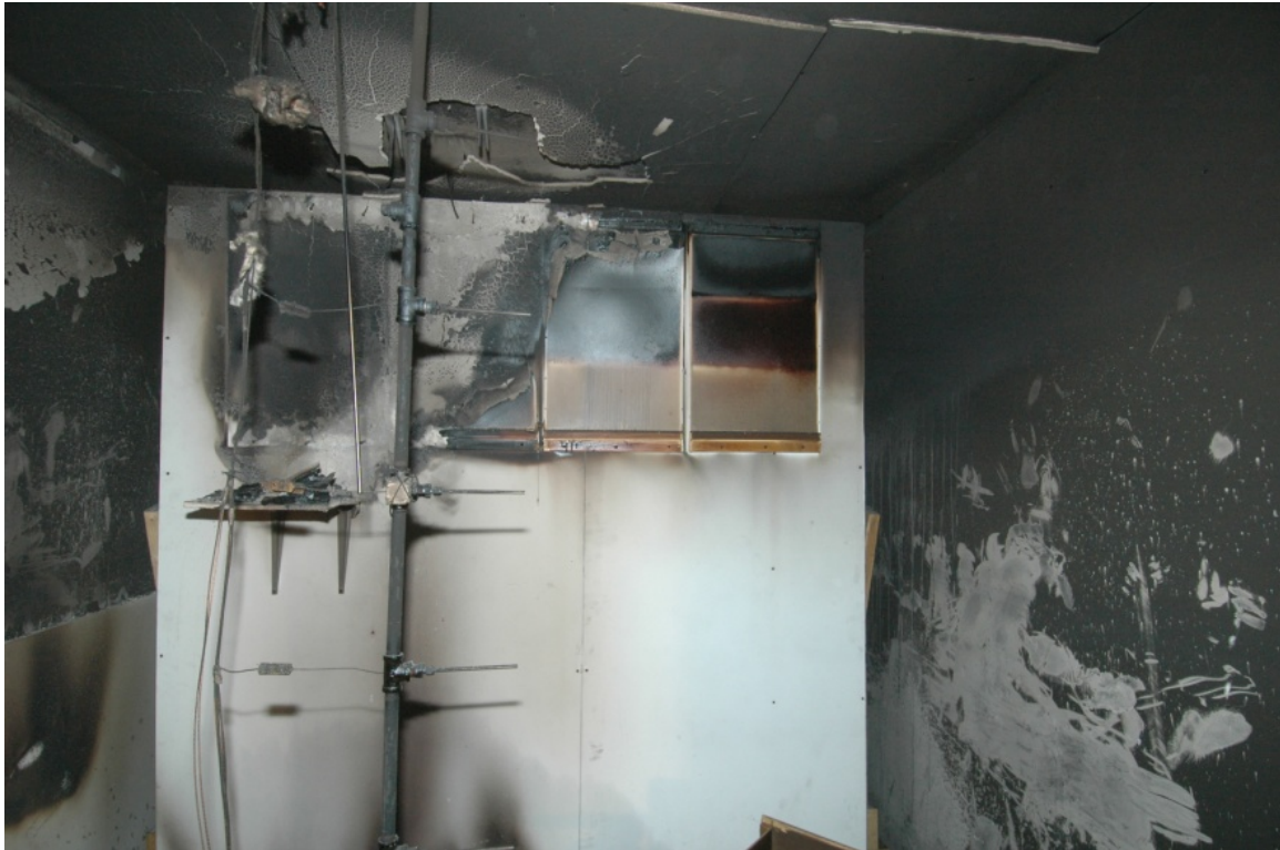
Figure 8-12. Fire pattern from test CH2 (half open window)
