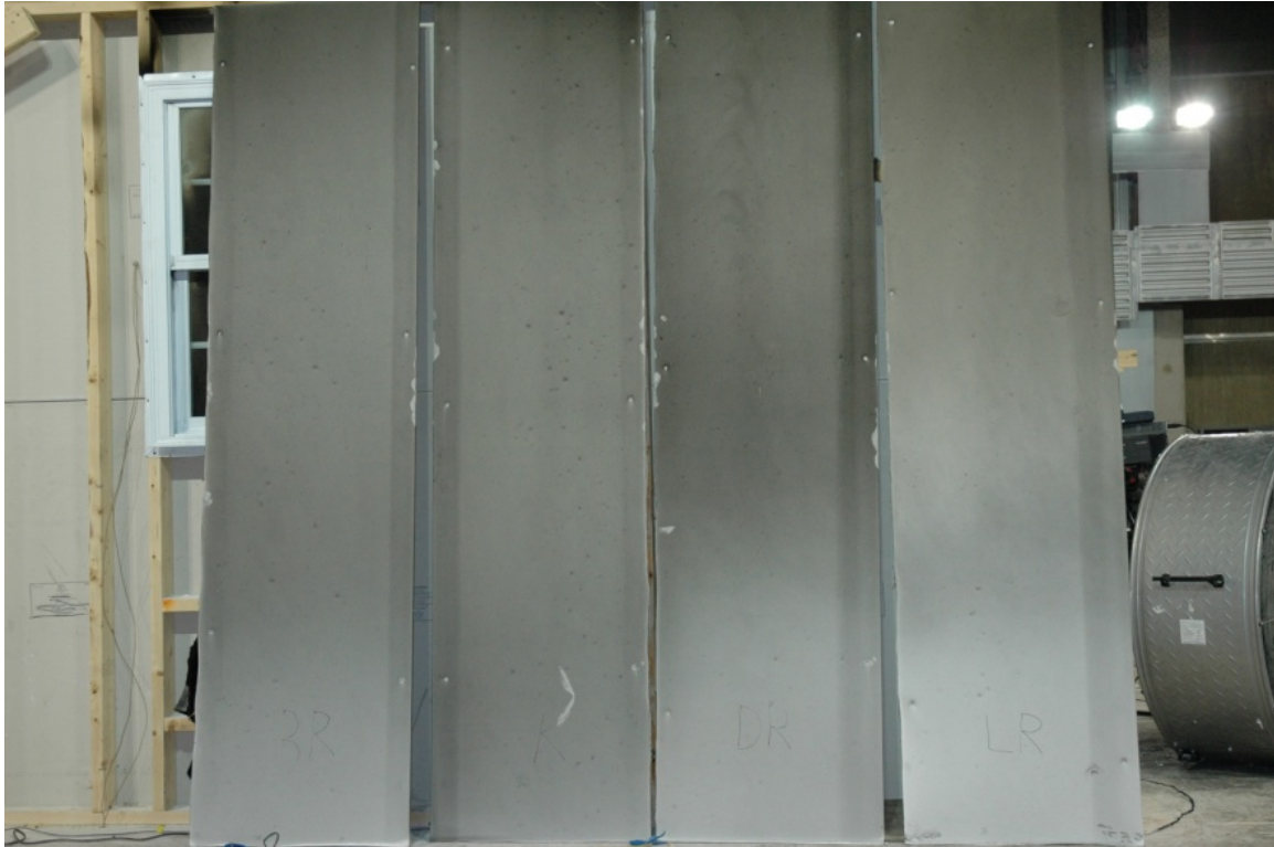
Figure 8-24. Test S3 (half open window) GWB targets (BR, K, DR, LR)
