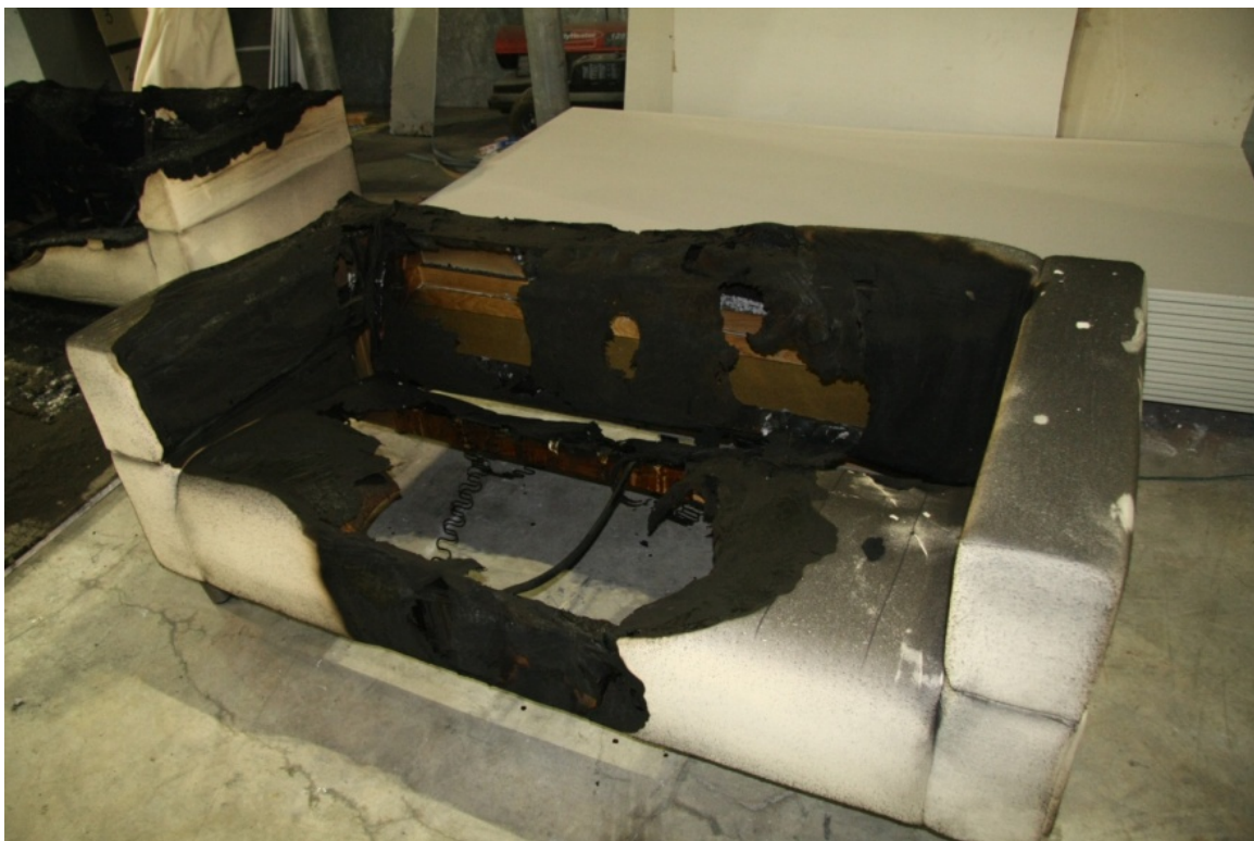
Figure 8-18. Sofa after test S4 (half open window accelerated)
