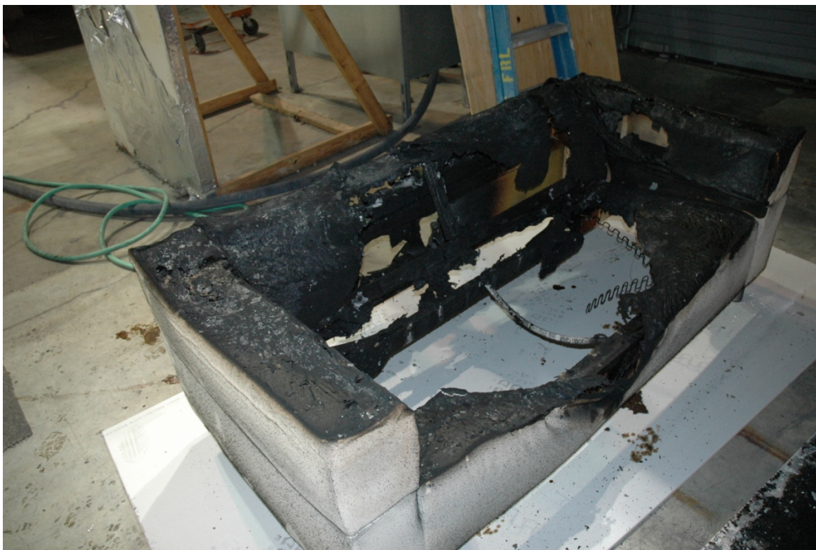
Figure 8-16. Sofa after test S3 (half open window)
