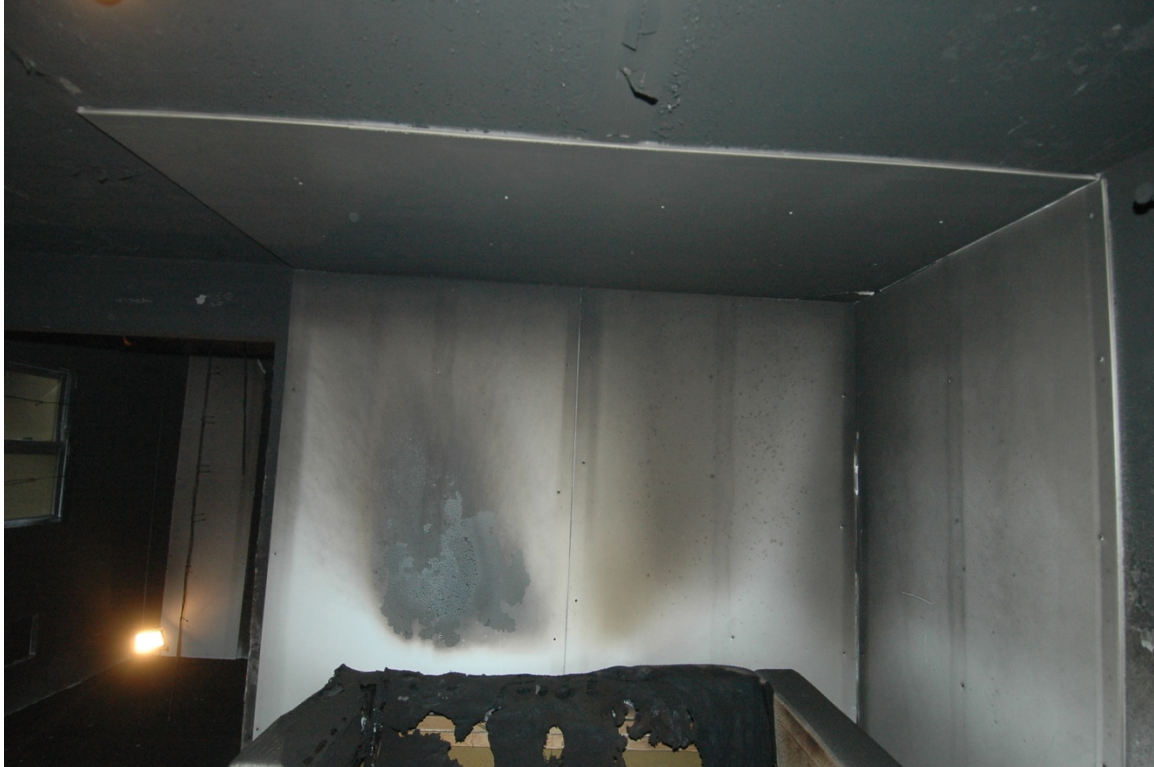
Figure 8-4 Fire Pattern from test S4 (half open window accelerated)
