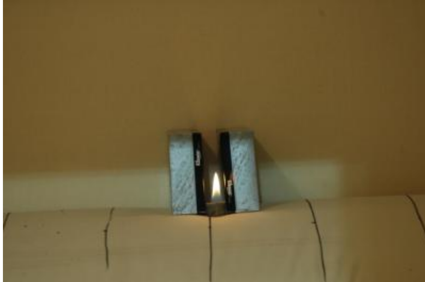
Figure 3-5. Accidental flaming ignition scenario setup
