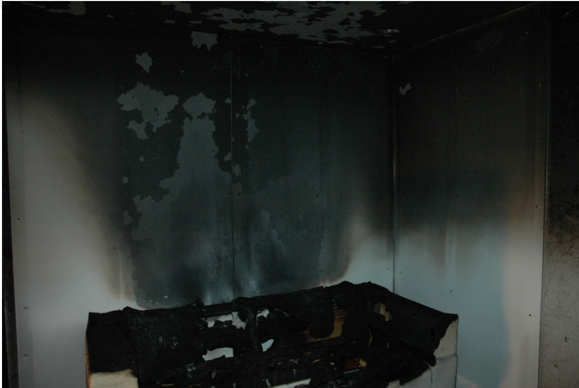
Figure 8-2. Fire pattern from test S3 (half open window)
