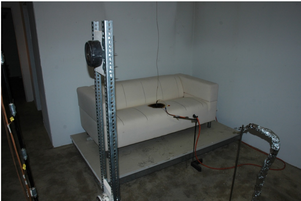
Figure 8-38. After smoldering sofa test (SM2 – no ventilation) (Note: this photo actually portrays the scene darker than observed on site due to the lighting in the space when the photo was taken.)
