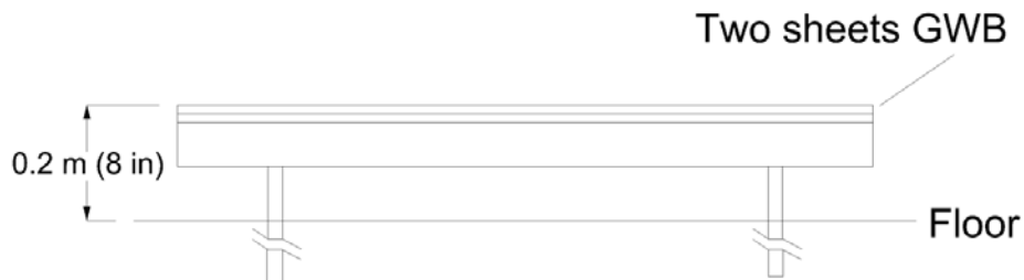
Figure 4-13. Side view of load cell frame inside enclosure
