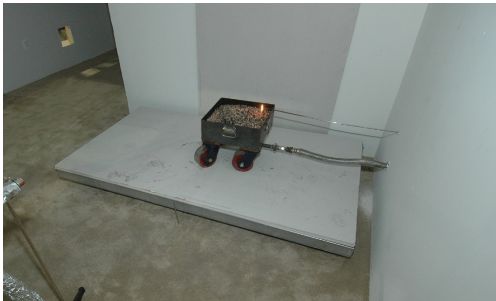
Figure 5-6. Burner placement for tests B1 and B2
