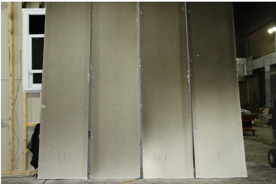
Figure 8-25. Test S4 (half open window accelerated) GWB targets (BR, K, DR, LR)
