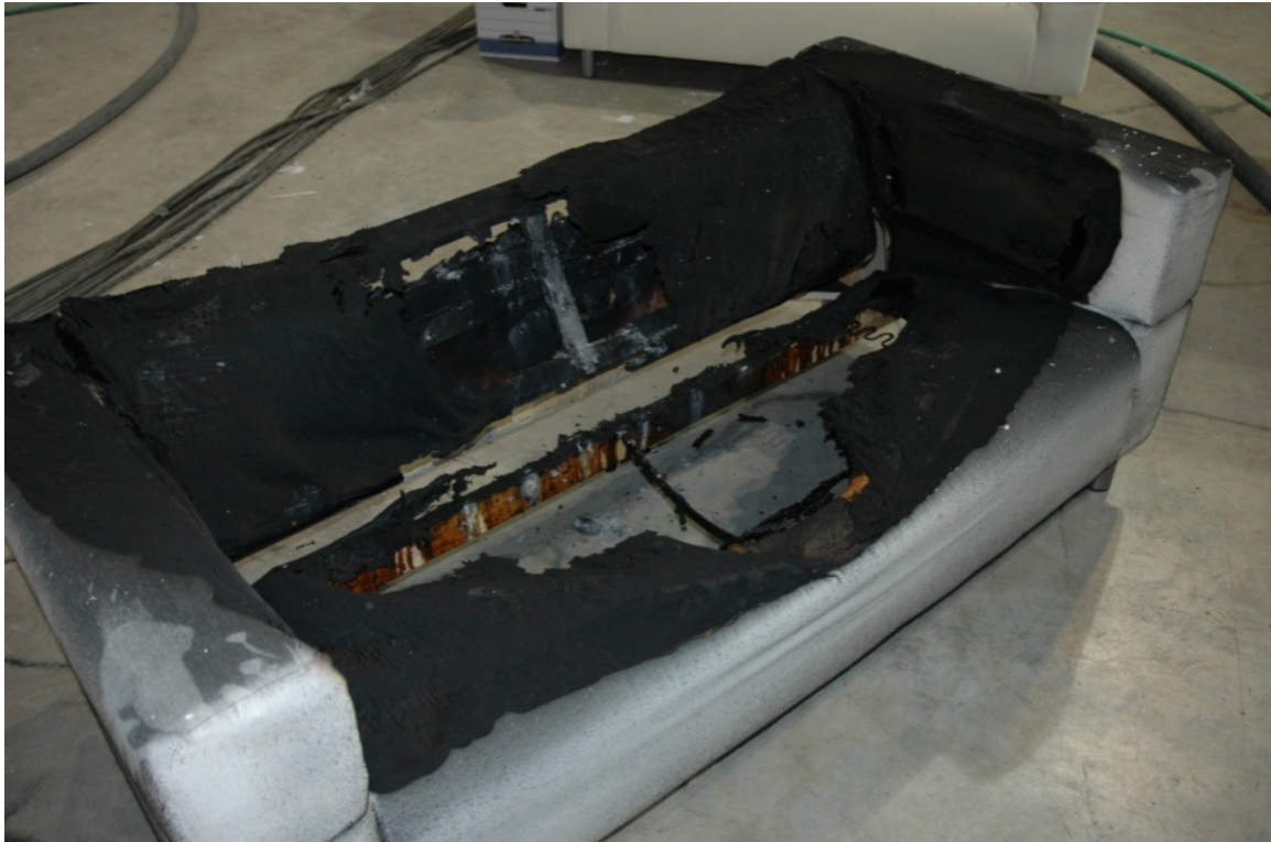
Figure 8-15. Sofa after test S1 (no ventilation)
