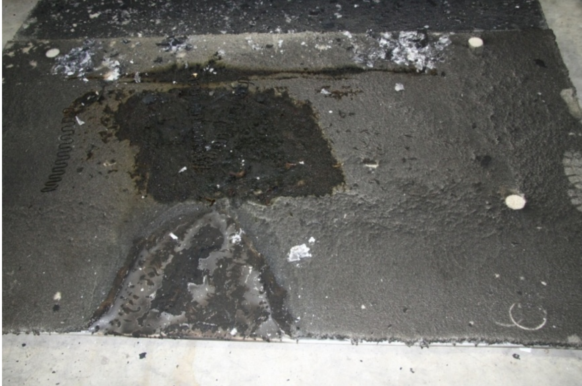
Figure 8-7. Burn pattern under and in front of sofa during accelerated test
