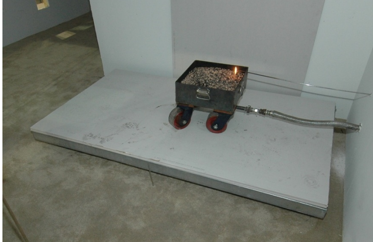
Figure 4-12. Mass loss frame in place during burner test
