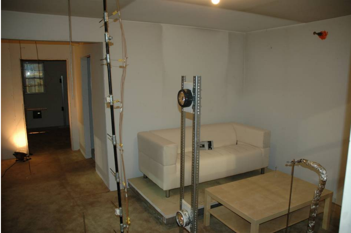
Figure 8-35. Before flaming sofa test (S1 – no ventilation)
