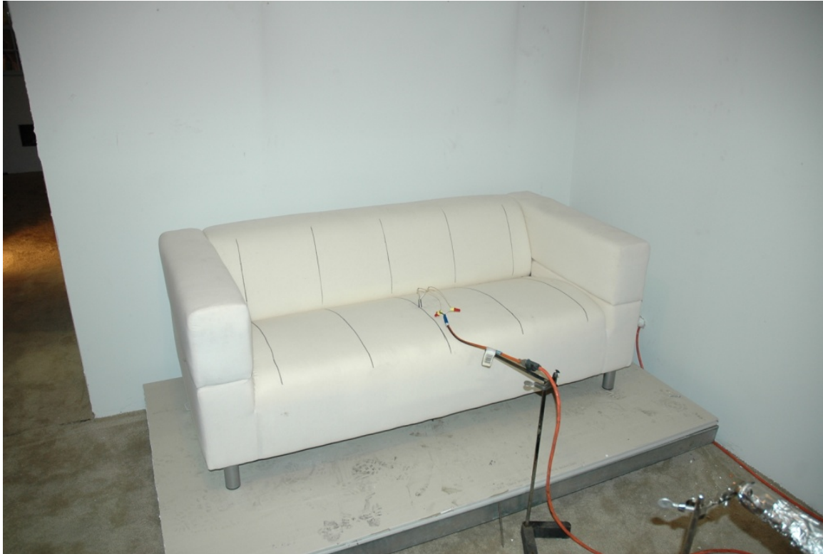
Figure 8-37. Before smoldering sofa test (SM2 – no ventilation)
