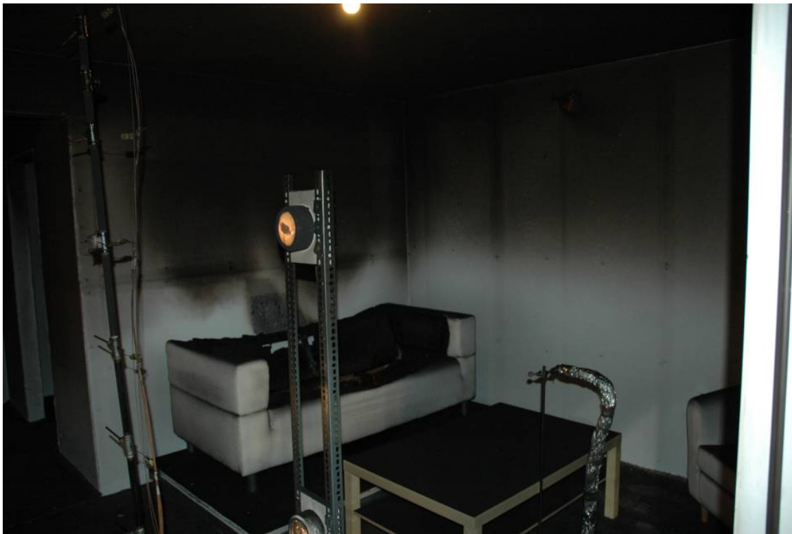
Figure 8-36. After flaming sofa test (S1 – no ventilation)
