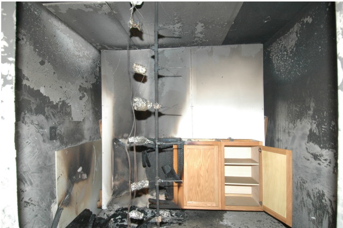
Figure 8-9. Fire pattern from test CL2 (half open window)
