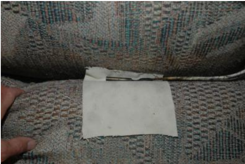
Figure 5-20. Cartridge heater setup for test SM4
