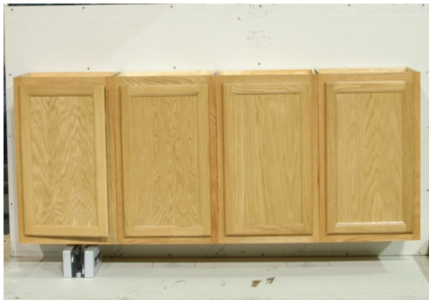
Figure 3-3. Cabinet array with ignition source
