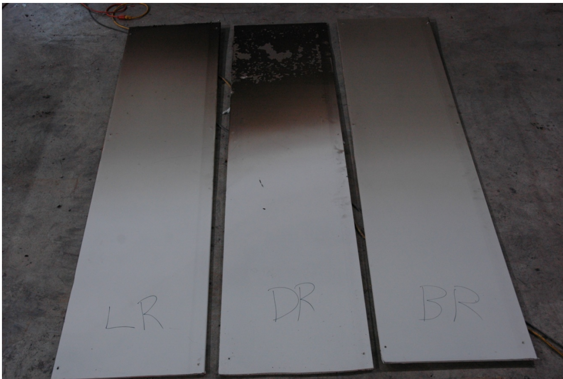
Figure 8-31. Test CL3 (open door) GWB targets (LR, DR, BR) (K target was destroyed during test)
