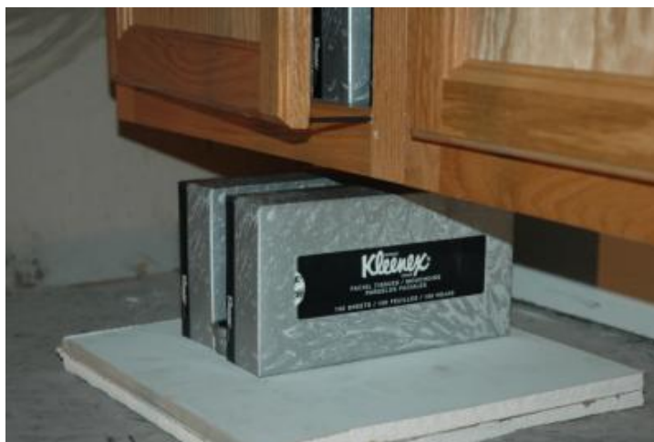
Figure 5-32. Ignition scenario for low cabinet flaming tests
