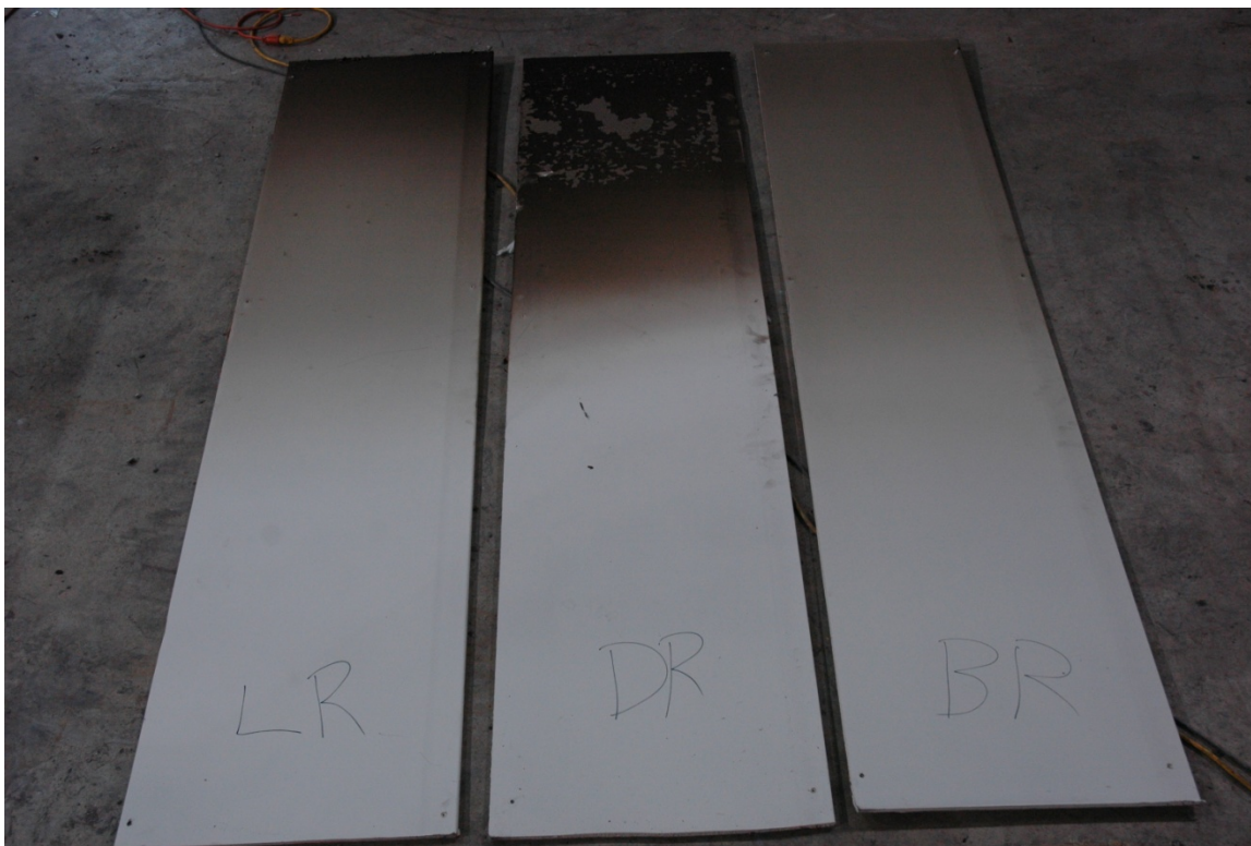
Figure 8-34. Test CH 4 (open door) GWB targets (LR, DR, BR) (K target was destroyed during test)
