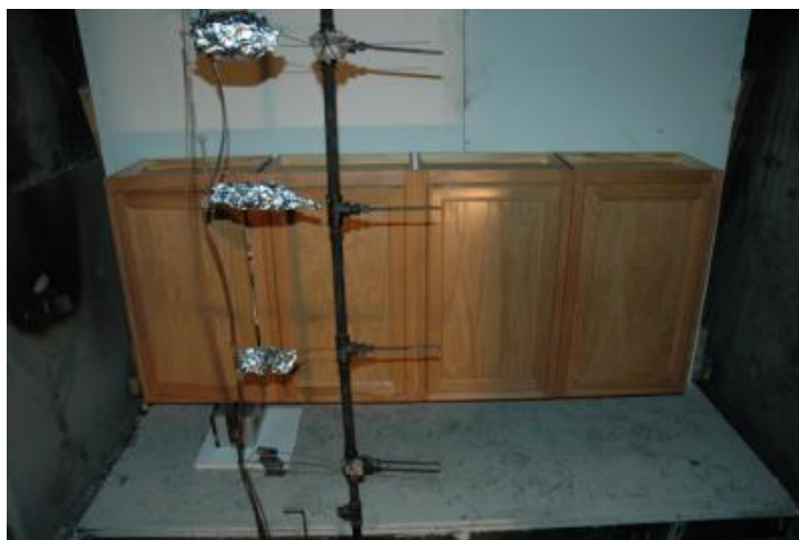
Figure 5-31. Setup for low cabinet flaming tests
