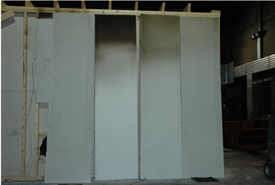
Figure 8-32. Test CH1 (no ventilation) GWB targets (BR, K, DR, LR)
