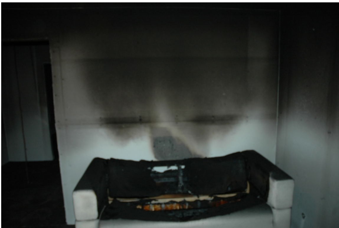
Figure 8-1. Fire pattern from test S1 (no ventilation)
