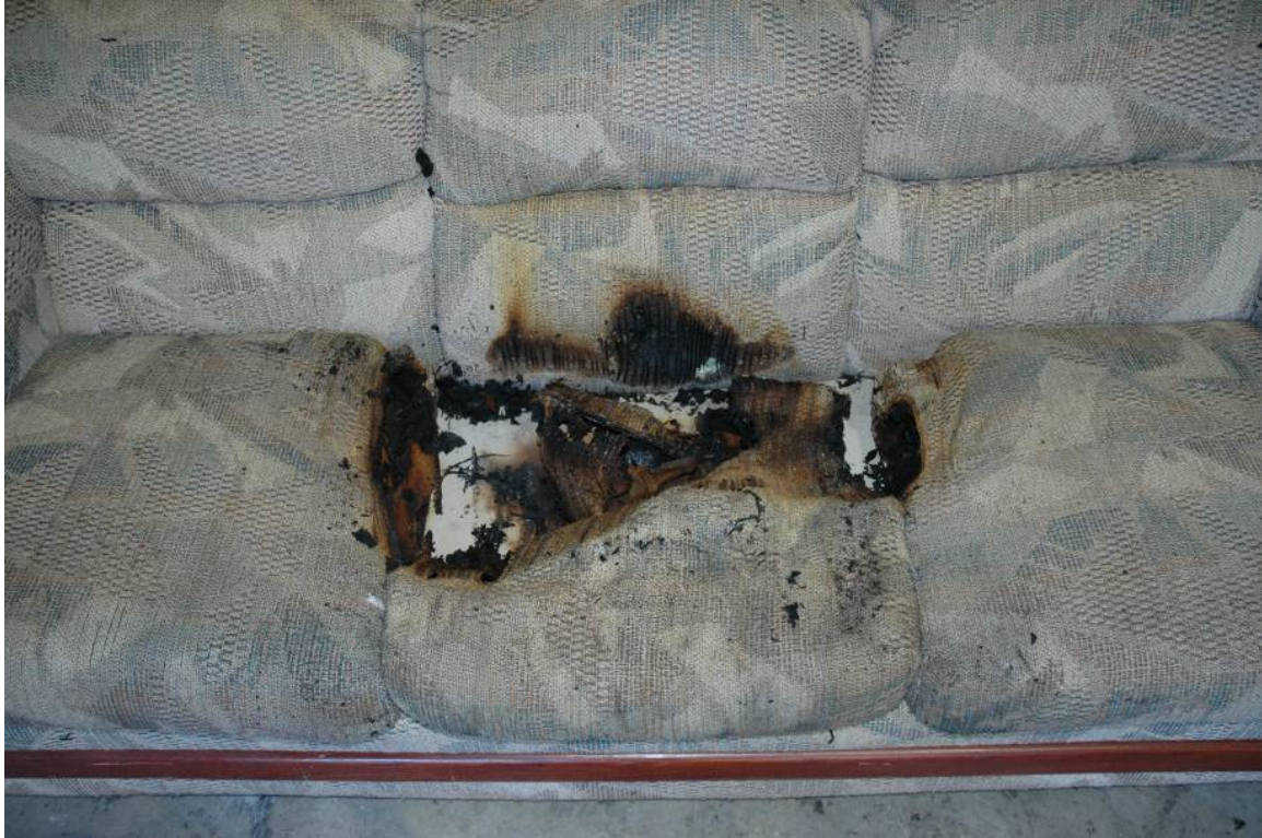
Figure 8-39. Damage to sofa after smoldering test (SM4 – no ventilation)
