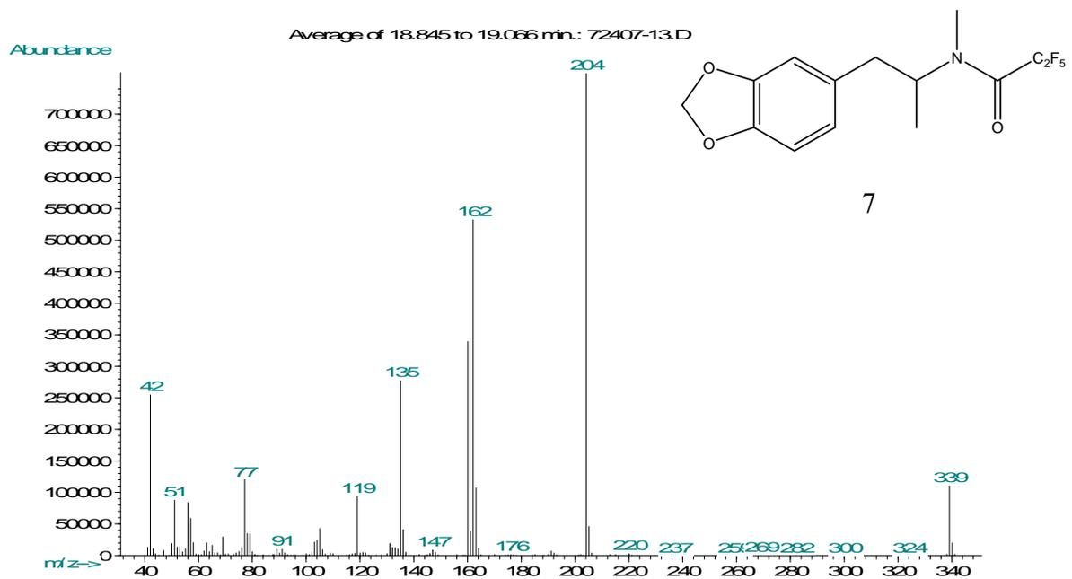
**Figure 3.4: Mass spectra of the HFBA derivatives of compounds 2-7.**
