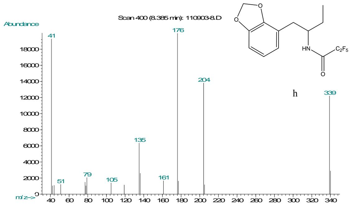
**Figure 1.3: Mass Spectra for the HFBA derivatives of compounds (2-5) and (7-10).**
