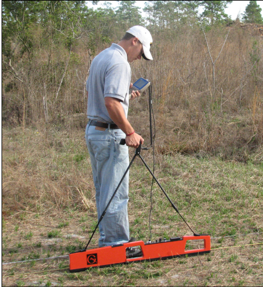
Figure 8: Operation of EMI meter in vertical dipole orientation by Michael Martin
