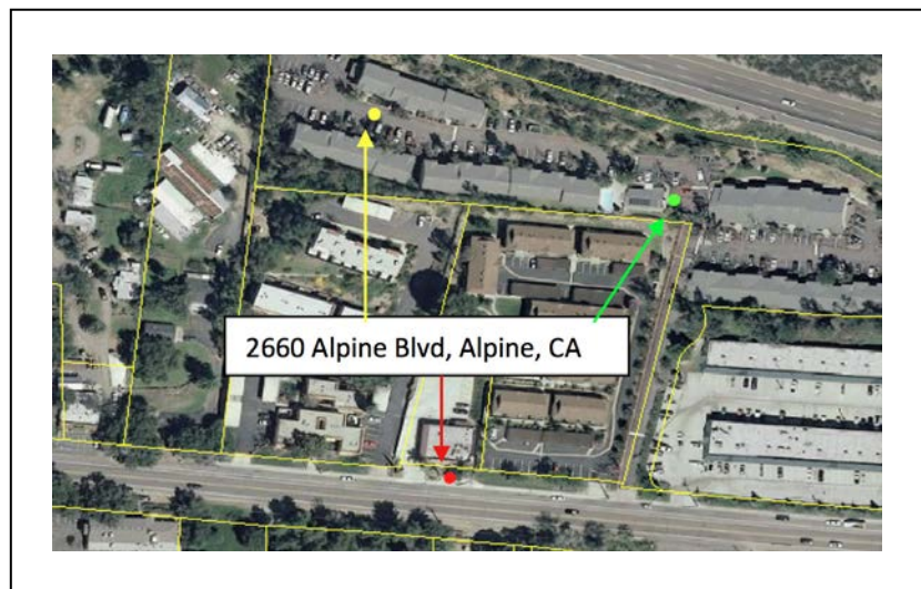
Figure 5. Illustration of an input address geocoded to three different reference layers. The red dot represents an address location geocoded against a street centerline file. The green dot represents the same address geocoded to a parcel centroid file, and the yellow dot represents the same address geocoded against address point reference data.
