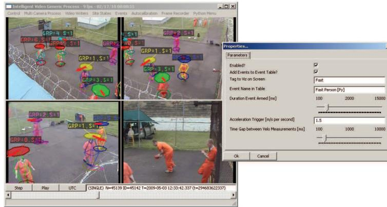
Figure 34: **Dynamic Event Detector Scripts:** Event detection algorithms can now be integrated in Python, a script-based programming language.
