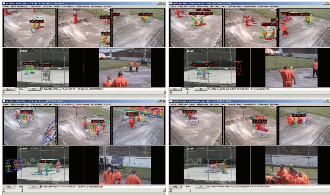
Figure 6: **Aggression Scenario.** Events detected live by the system during an aggression scenario enacted by Lake Erie Corrections. The aggression in the last frame is indicated by the red rectangle that is partially hidden by an overlaying loitering label.
