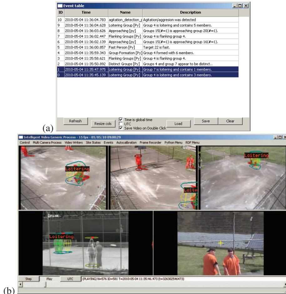
Figure 54: **Loitering event:** (b) Screen shot of our system detecting a loitering event: (a) The detected loitering event is stored in the event table. (b) The screen shot of the detected loitering event. The screen short shows an enactment by Lake Erie correctional officers.
