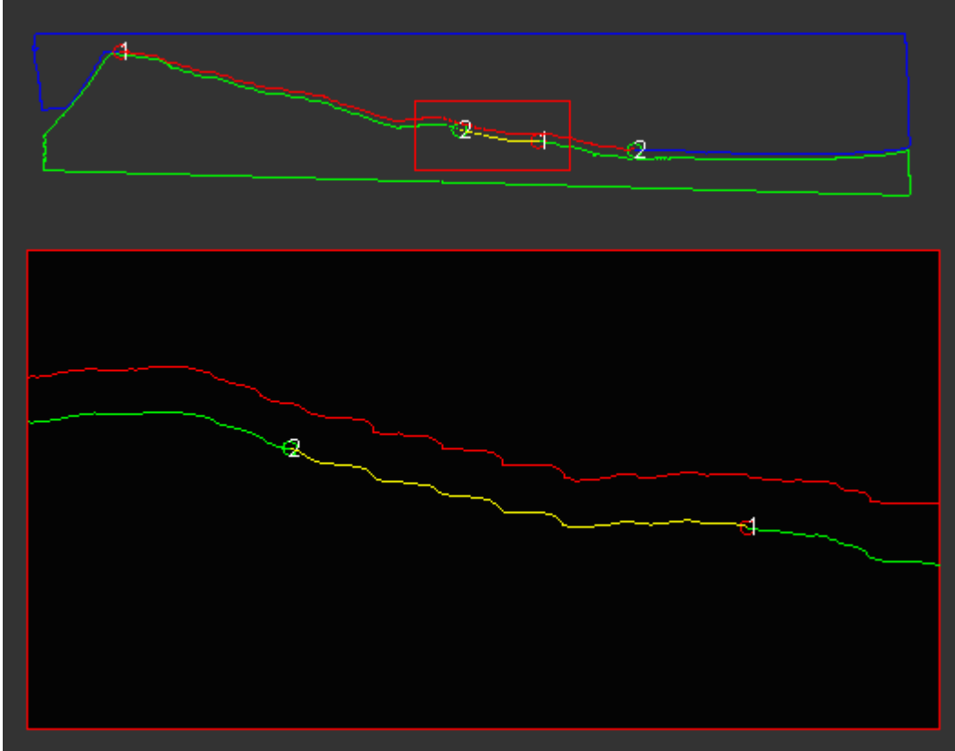
Figure 3. Choosing the target and search area. The two contours are displayed simultaneously in two views: a zoomed out view of the entire contours (top) and a zoomed in view, magnifying a specific feature (bottom). The red rectangle on the top view marks the area that is magnified on the bottom view. The user marks the search area on the top contour using two points (red and green circles). The search area is the red part on top of the blue contour. Setting the borders of the area is done by moving the mouse cursor to the desired location and then pressing the “1” or “2” keys. The same method is used on the bottom contour to mark the target which is displayed as a yellow part on top of the green contour. The user can change the scale of the bottom view (zoom in and out) and move and rotate one contour with respect to the other to be able to finely choose the target and search area.
