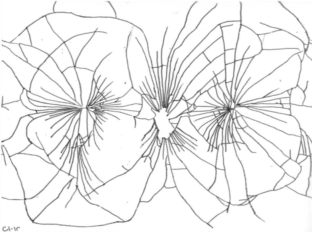
Figure 16 Fracture pattern using round impact tip
