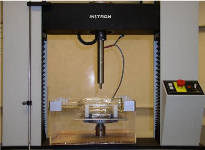
Figure 8 Instron® 4204 Tensile Tester (glass bottle setup shown)
