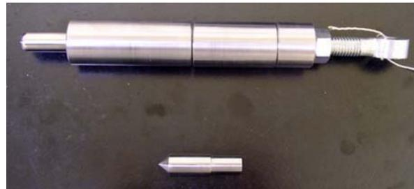
Figure 2 Dropping weight with interchangeable impact tips (round and sharp shown)
