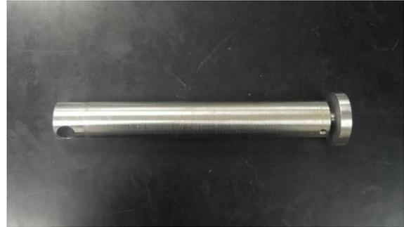
Figure 9 Indenter with wide fracture tip (right side)
