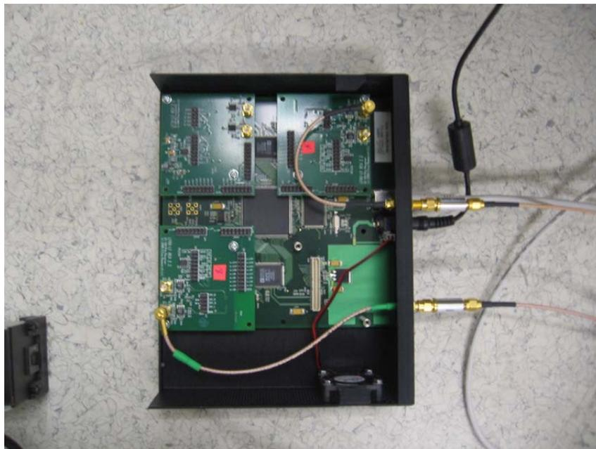
**Figure 74. USRP data acquisition system.**
