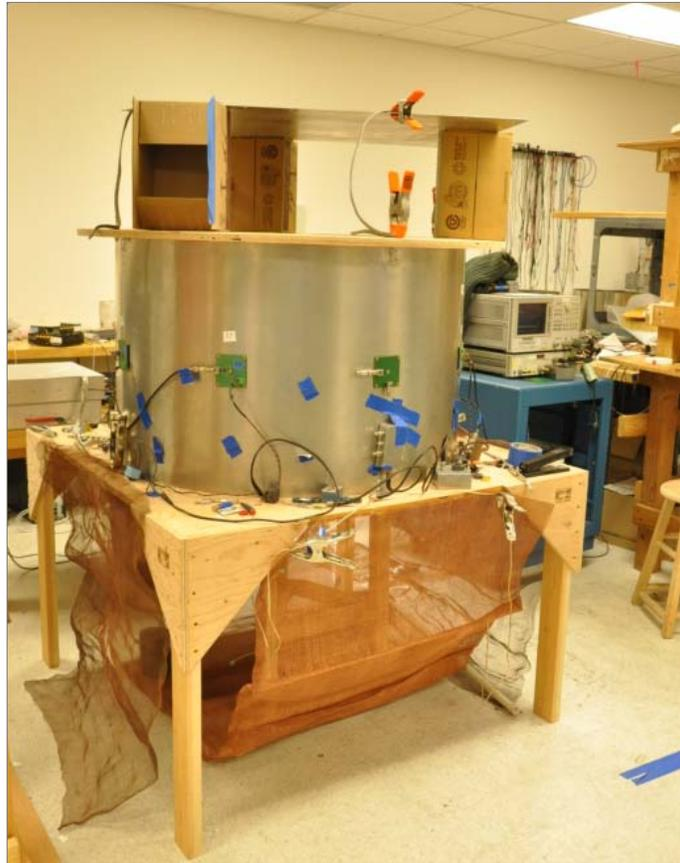
Figure 89. EFT system being tested with additional shielding.
