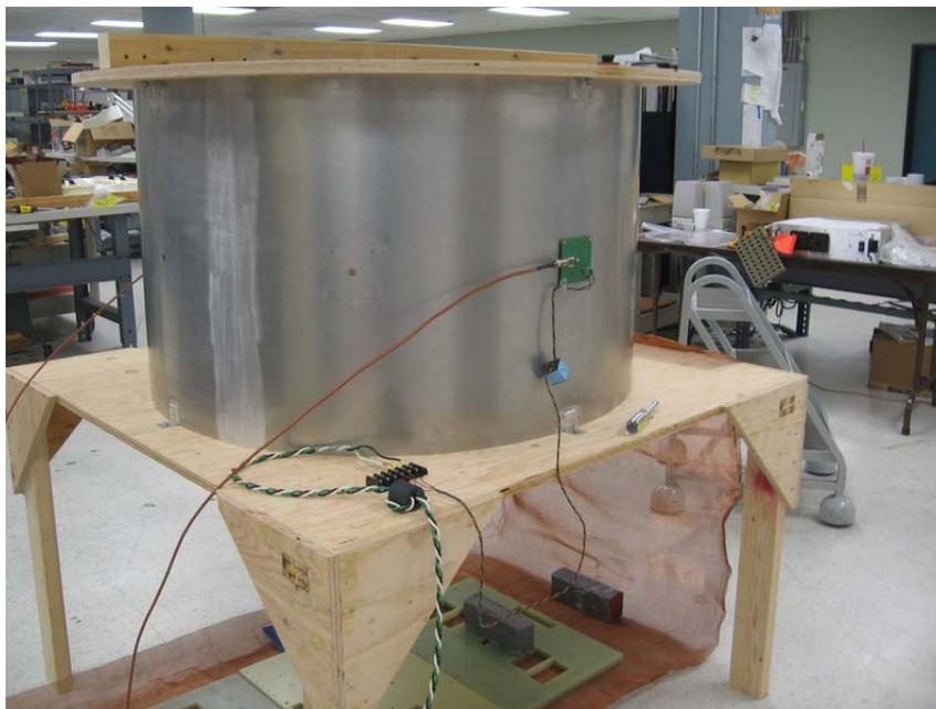
**Figure 70. Shield for prototype system with attached receiver board.**
