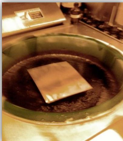
Figure D2: Copper substrate positioned within rotating machine tub after application of the photoresist.
