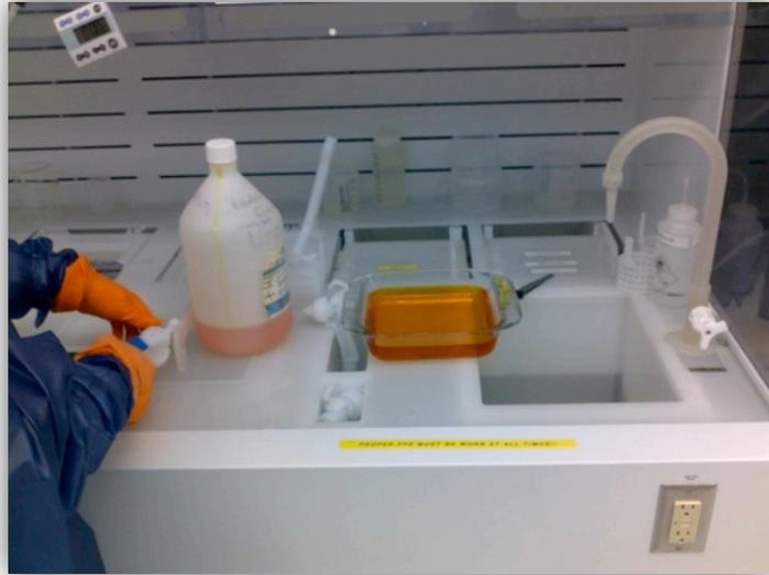
Figure D6: Ferric Chloride used for etching the copper clad laminate in the clean room.
