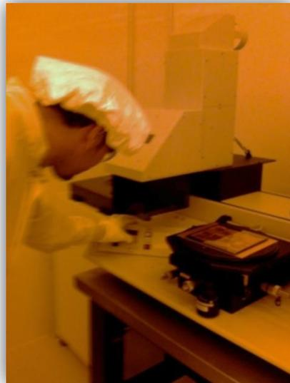
Figure D4: Glass photomask aligned over the photoresist coated copper substrate prepared for UV exposure.
