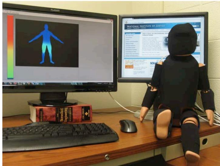
Figure 11. Surrogate bruising detection system: ATD equipped with sensing skins and 3D body image map illustrating activated sensors.
