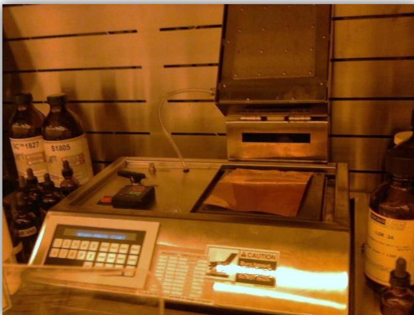
Figure D3: Photoresist coated copper substrate placed on the hot plate for soft baking.
