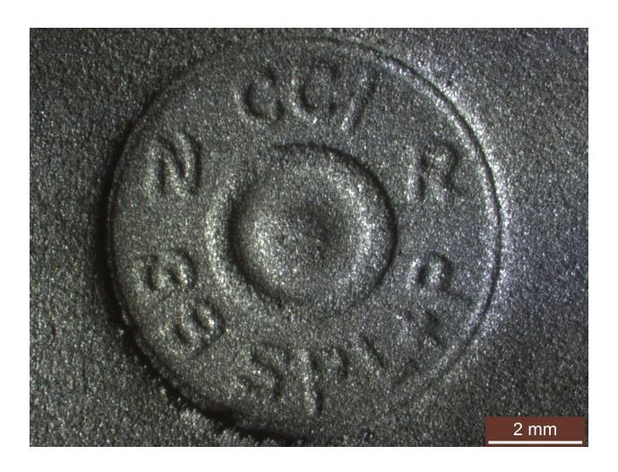
4. Figure 4 – This image displays the effect of using an MR fluid in which the iron particles have begun to oxidize. The image shows the original impression artifact for comparison. There are also MR fluid remnants clearly visible on the original artifact.
