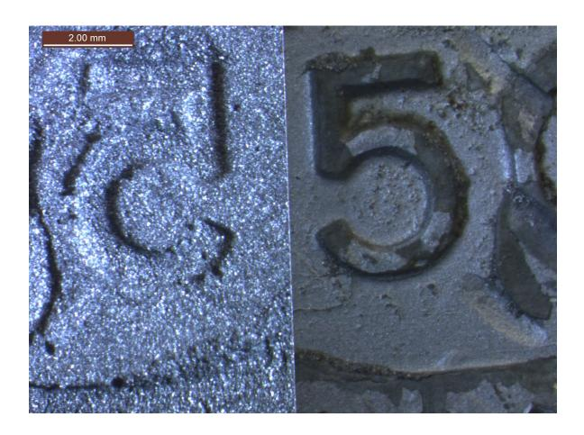
6. Figure 6 – This image highlights the level of detail achievable using MR fluids as a casting agent. A unique mark was made on the "N" of the bullet casing, in order to give the researchers a way to judge the resolution of the trial MR fluids. Using the optimized fluid formula, MRF.W#10, a cast was made. The scale indicates that the fluid is able to capture fine details down to approximately 0.2mm in size. The image has been flipped vertically for ease of visualization.
