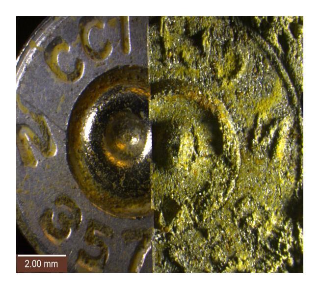
5. Figure 5 – This image displays a zoomed in side-by-side comparison of the "5" ridge of a 500 gram weight and the impression it left in a cast made with MRF.W#10. The image shows that impressions on the sub-millimeter level may be retained with MR fluids.
