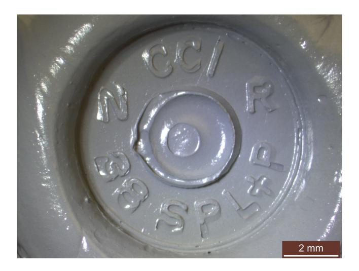
3. Figure 3 - This photograph contains a cast made of the bullet shell casing in Figure 1, made with the optimized MR fluid formula, MRF.W#10. The image is horizontally flipped in order to be more easily comparable to the original impression artifact.
