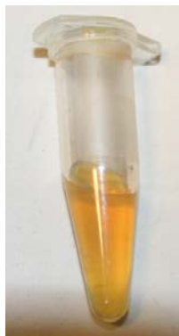
Figure 2. Ag colloid synthesized by microwave reduction.
