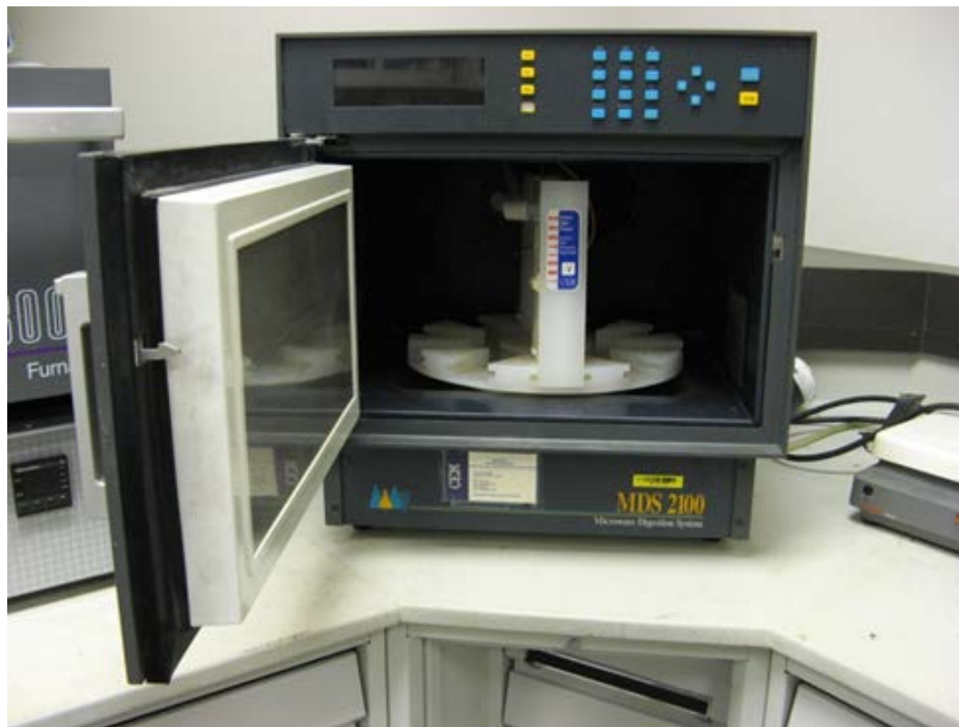
Figure 1. The CEM MDS-2100 microwave digestion system with a pressure resistant Teflon microwave vessel where the nanoparticle synthesis is carried out.
