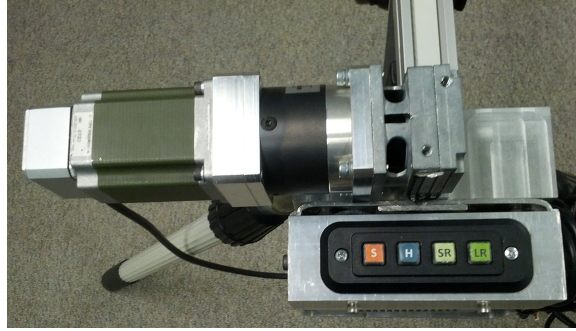
Figure 18: Four button control pad of the device.
