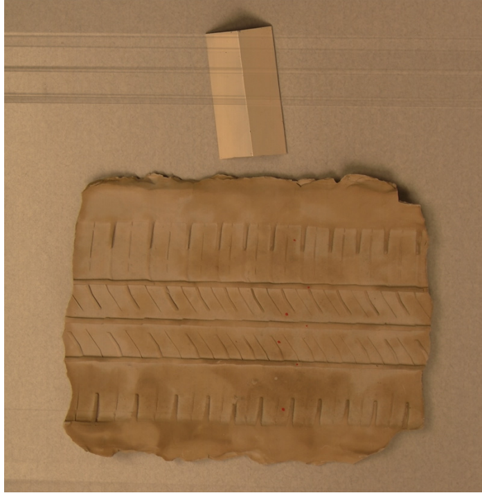
Figure 26: This color texture image is generated by stacking frame stripes (1 pixel thick, horizontal stripes). Furthermore, it is registered with the computed height maps.
