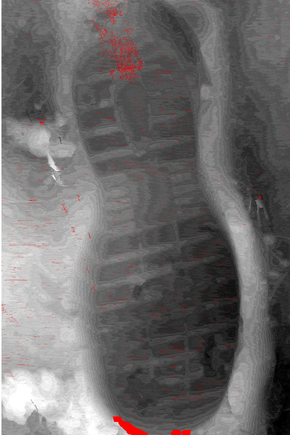
Figure 31: z range: 305.5mm, 256.0mm. The red pixels indicate locations where we do not have laser data to compute depth values. Brightness indicates height values—the brighter the value the closer the point on the surface is to the cameras optical center (i.e., the larger the height).
