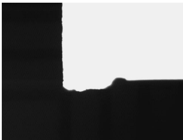
Figure 15: Inner edges were not always straight and abrasions were frequent, making them inadequate for measuring perpendicularity. The above is an example of small imperfections caused by the cutting of rulers in the manufacturing process.
