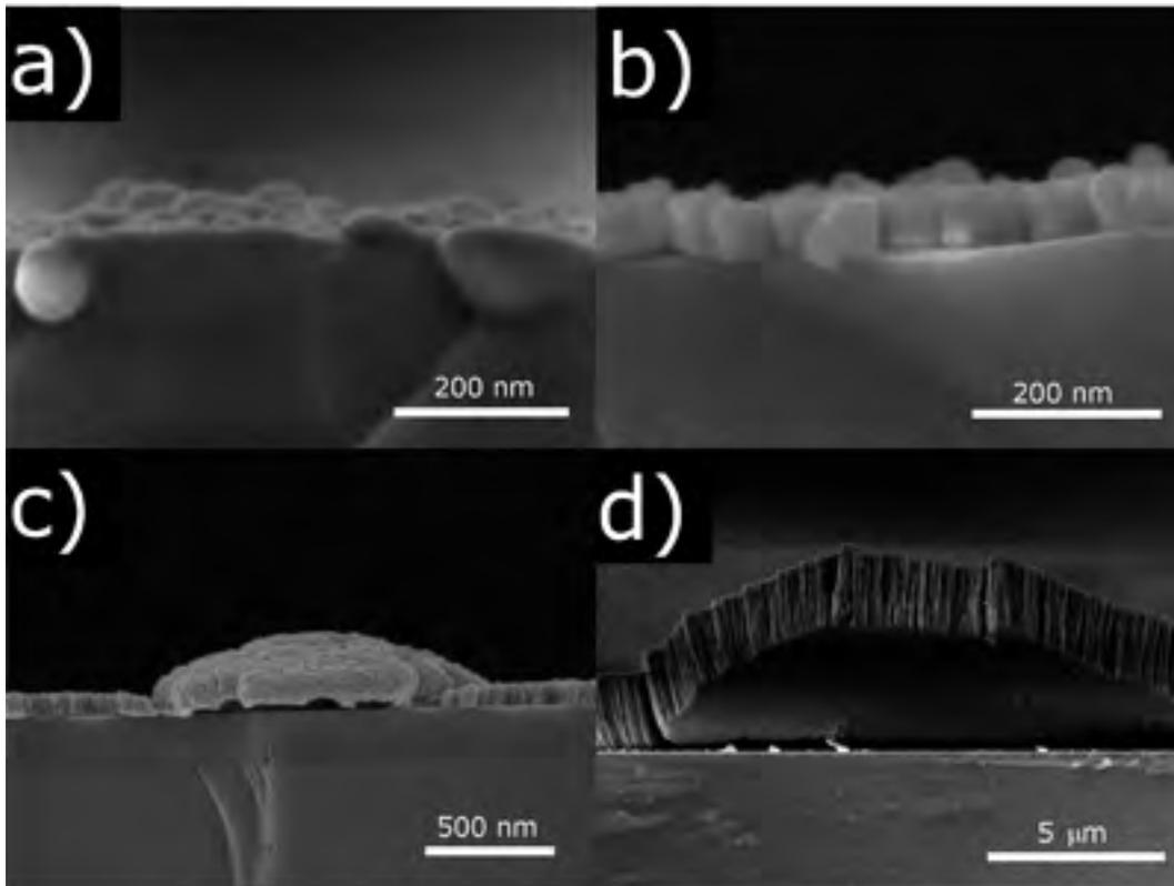
FIG. 26—Cross-sectional SEM images of (a) a zinc film deposited atop a gold film on a fingermarked silicon substrate by VMD, (b) a gold CTF deposited on a planar silicon substrate by the CTF technique, (c) a fingermark ridge on a silicon substrate conformally coated with a nickel CTF, and (d) a fingermark ridge on a glass slide conformally coated with a chalcogenide-glass CTF.
