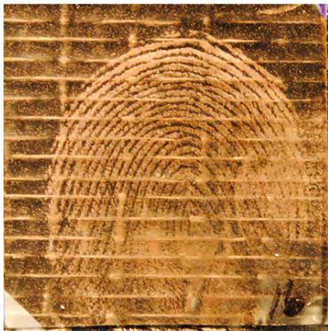
FIG. 4—Fingerprint on the smooth side of Scotch® Duct tape developed by a hybrid technique involving pretreatment of the latent fingerprint by cyanoacrylate fuming followed by the deposition of a 50-nm-thick CTF of gold.
