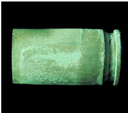
FIG. 22—Fingerprint on a bullet casing developed after discharge by a hybrid technique involving pretreatment of the latent fingerprint by cyanoacrylate fuming followed by the deposition of a 100-nm-thick CTF of Alq<sub>3</sub>. Short-wave ultraviolet illumination is needed to see the detail.
