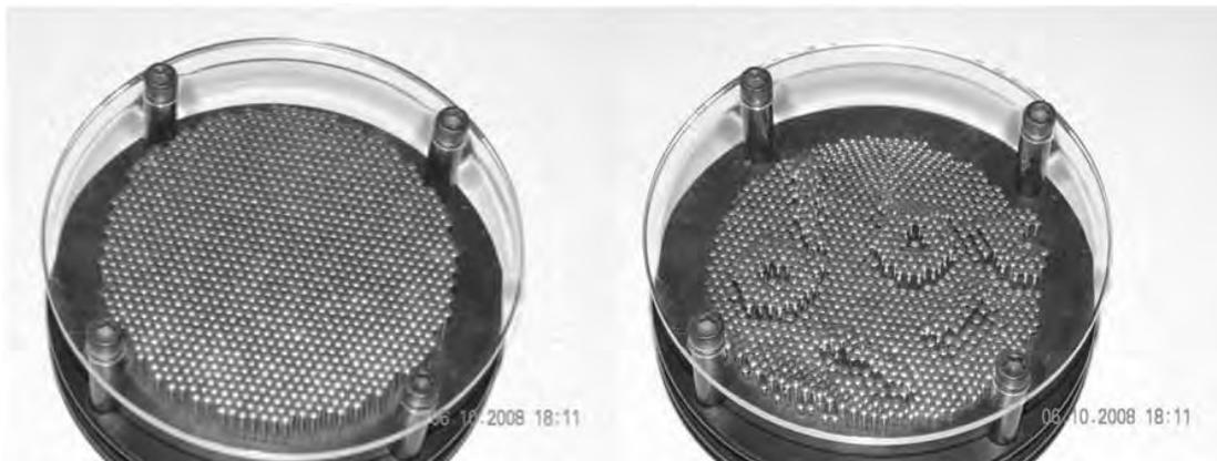
FIG. 1—Illustration of the CTF concept using a toy called Pin Point Impression comprising parallel, identical, thin cylindrical pins. Left panel: Pins over a flat surface. Right panel: Pins over an undulating surface.
