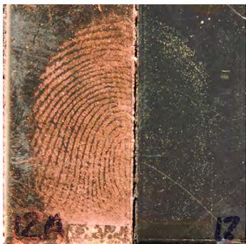
FIG. 16—Fingerprint on black nylon developed either (left) by the use of red fluorescent powder or (right) by the deposition of a 100-nm-thick CTF of Alq<sub>3</sub>. Short-wave ultraviolet illumination is needed to see the detail in the CTF-developed part of the fingerprint.
