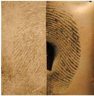
FIG. 11—Fingerprint on a black garbage bag (soft plastic) developed either (left) by the use of white magnetic power or (right) by the deposition of a 100-nm-thick CTF of nickel. Level-three detail is clearly seen in the CTF-developed fingerprint.
