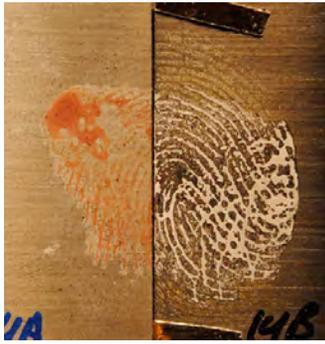
FIG. 20—Partial bloody fingerprint on 420-grade stainless steel developed either (left) by the use of cyanoacrylate fuming followed by dusting with regular black powder or (right) by the deposition of a 100-nm-thick CTF of nickel.
