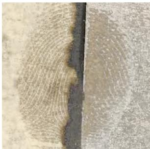
FIG. 10—Fingerprint on the sticky side of Scotch® Masking tape developed either (left) by the use of Wetwop™ or (right) by the deposition of a 100-nm-thick CTF of nickel.
