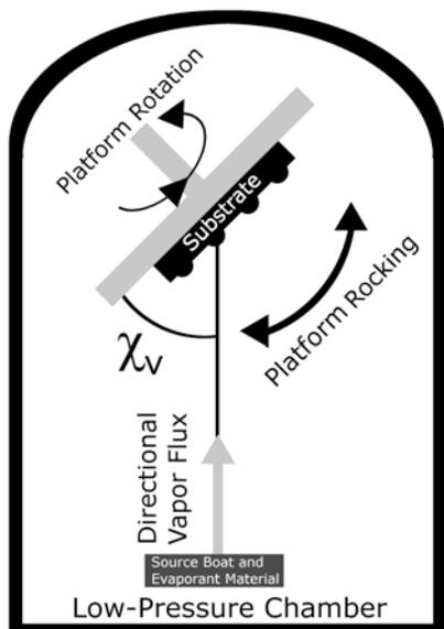
FIG. 2—Schematic of the CEFR method. In a low-pressure chamber, a collimated vapor flux is directed towards a substrate mounted on a platform that rotates rapidly about a central normal axis. The platform may also be made to rock slowly about an axis lying wholly in the platform plane so that the angle  $\chi_v$  between the average direction of the vapor flux and the platform plane varies periodically, provided the exposed surface of the substrate is significantly lenticular.
