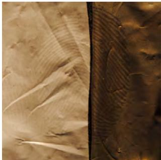
FIG. 13—Fingerprint on a white grocery bag (soft plastic) developed either (left) by the use of black magnetic power or (right) by the deposition of a 100-nm-thick CTF of nickel.
