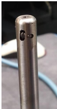
Photograph 1: EBIS tool with carbide steel cutting wheel.
