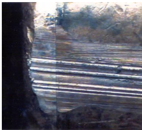
Photograph 2: Photomicrograph of the EBIS pattern on two fired bullets.
