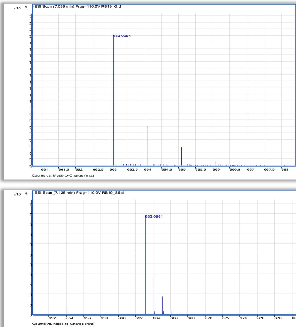
Figure 22. Comparison of the mass spectrum corresponding to the diode array peak at 7.10 min for the synthesized Reactive Blue 19 with glucose (Top) and Reactive Blue 19 extracted from cotton sample (Bottom).
