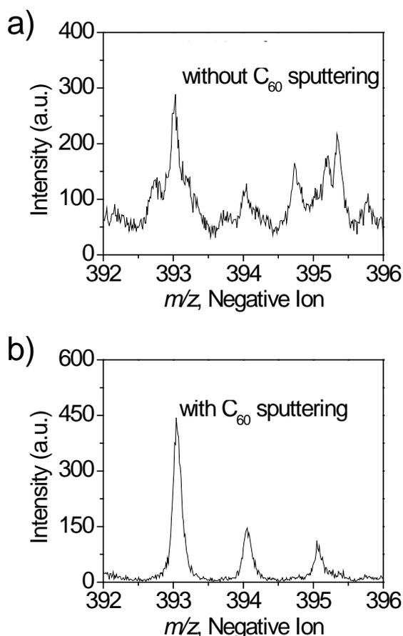
Figure 8. Negative ion TOF SIMS spectra obtained from 0.5% owf Acid Blue 25 dyed nylon surface (a) without  $C_{60}$  sputtering, and (b) with  $C_{60}$  sputtering for 14.6s at 1 nA followed by spectrum acquisition with  $Bi_3^+$  at 1 shot/pixel for 20 frames with this cycle repeated 30 times. Both spectra (a) and (b) are reconstructed from 600 frames of 128 x 128 pixels, 1 shot/pixel  $Bi_3^+$  data acquisition.
