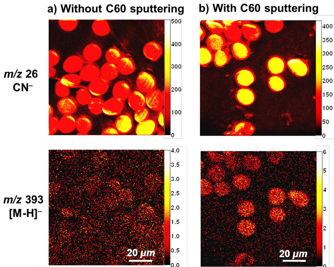
Figure 10. TOF SIMS images ( $100\ \mu\text{m} \times 100\ \mu\text{m}$ ,  $256 \times 256$  pixels, 1 shot/pixel) of 0.1% owf Acid Blue 25 dyed nylon cross section a) acquired with  $\text{Bi}_3^+$  beam only and b) acquired with  $\text{C}_{60}$  sputtering. The total acquisition was 600 frames.
