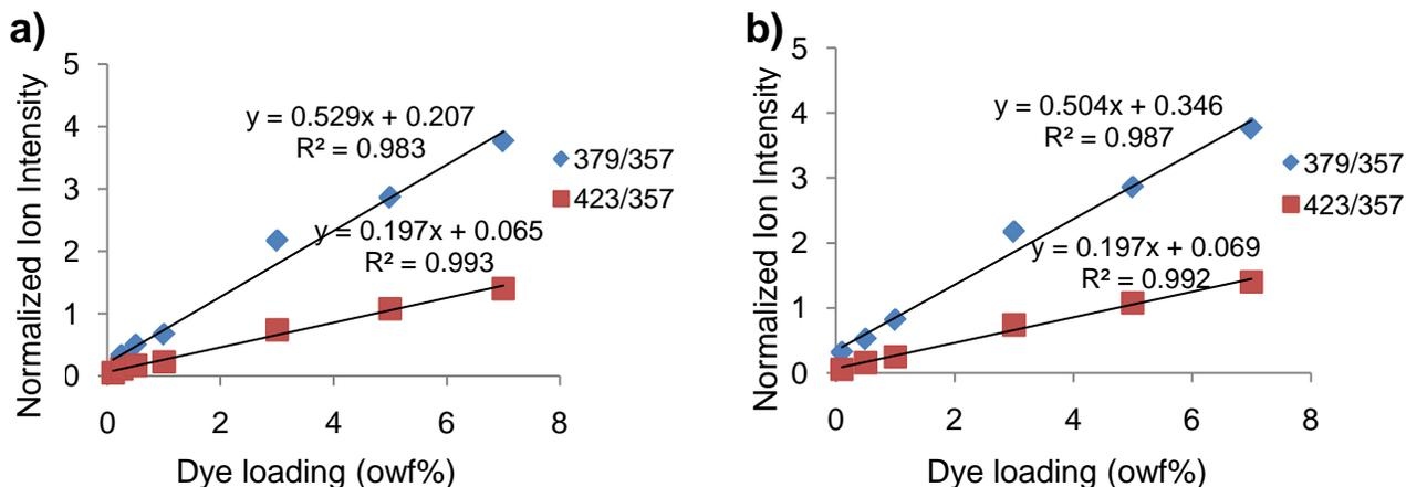
Figure 4. Normalized Disperse Blue 60 molecular ion ( $m/z$  379 and  $m/z$  423) secondary ion intensities versus dye loading obtained from cryomicrotomed fiber cross sections are presented. (a) The first set of Disperse Blue 60 dyed fabric cross-sections analyzed. (b) The second set of Disperse Blue 60 dyed fabric cross-sections analyzed.
