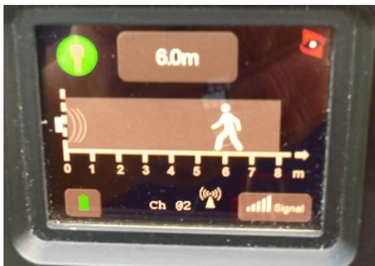
Figure 5: Xaver 100 Pre-Production Model Normal Mode Display Photo by NLECTC SSBT CoE
