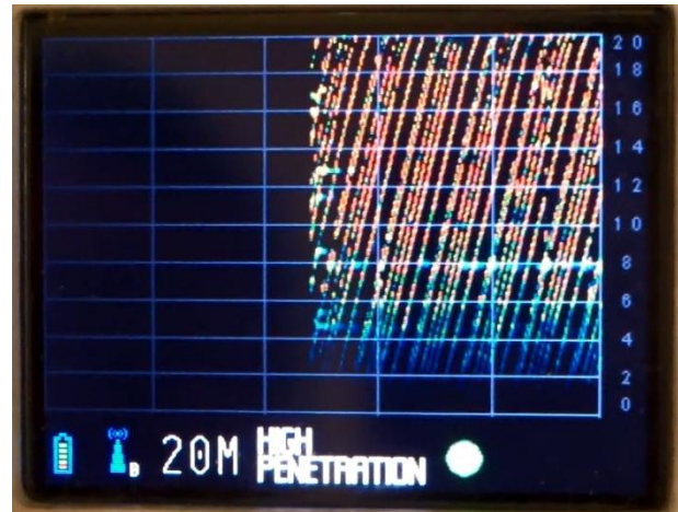
Figure 20: Xaver 400 – DWMS: ATW (HP) Difficult to make out target standing sideways at 8 m in High Penetration mode Photo by NLECTC SSBT CoE
