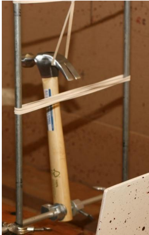
Figure 1 Hammer set to be propelled by rubber band on to a wooden block to create blunt force impact spatter (Method 1).
