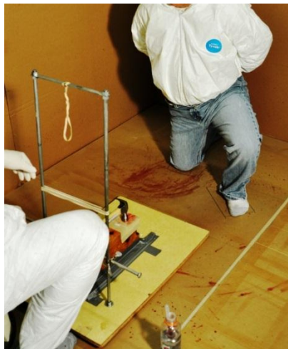
Figure 12 Preparation of blunt force impact spatter patterns on fabric surfaces
