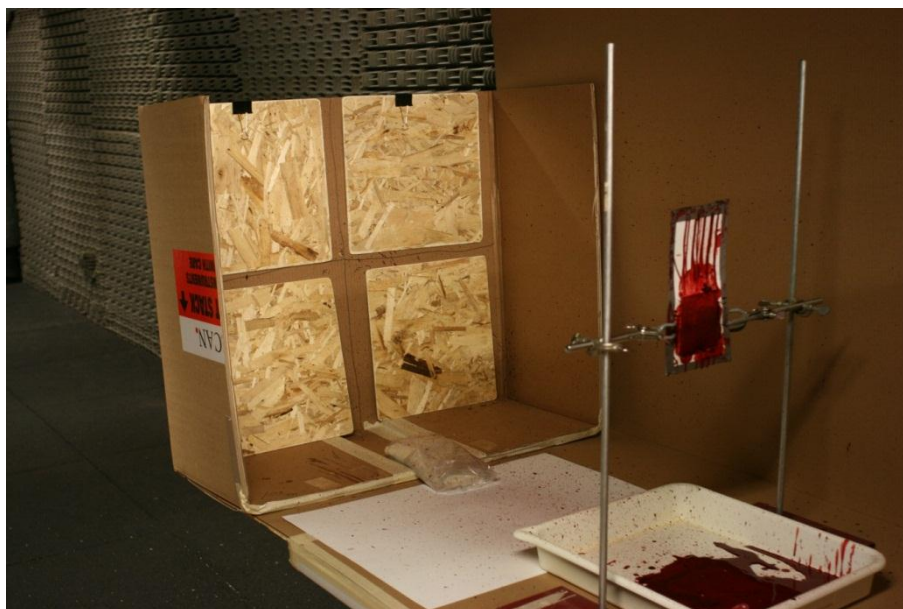
Figure 2 Blood soaked sponge and target arrangement to create forward spatter for firearms-related spatter patterns (Method 2).
