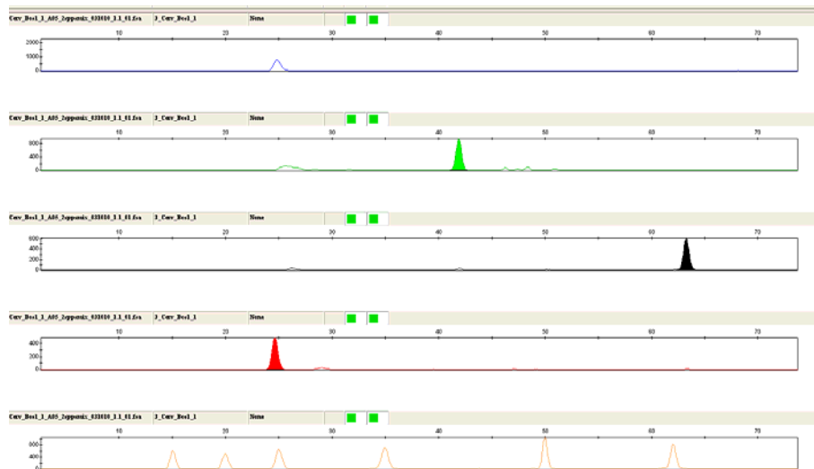
Figure 11. Electropherograms from SBE mini-primer sets 1 (a) and 3 (b) for a two species mixture of deer and cow DNA. Four clear peaks can be seen corresponding to 13F (64 red in set 1); 7R (42 green in set 3); 980F (63 black in set 3); and 841F (24 red in set 3).
