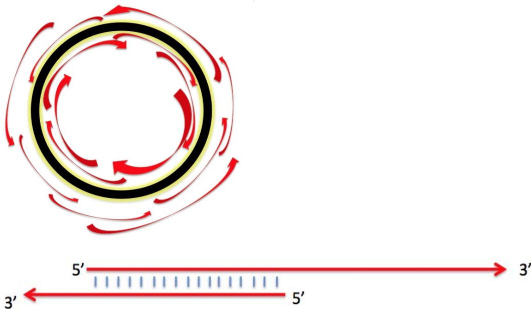
*Figure 21 – Stylized depiction of the expected products from an mtDNA-based whole genome amplification reaction. Top – circular view, bottom – linear view. These partially double stranded products should serve as templates for limited whole genome amplification, providing sufficient template for whole mt-genome analysis.*
