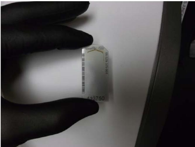
*Figure 3: The Pico Titer Plate (PTP) is the platform on which the DNA capture beads are immobilized in the Roche GS Junior™, and the location of the sequencing reactions and data collection. It houses a honeycomb of wells sized to hold a single DNA capture bead. Each sequencing run consumes a non-reusable PTP.*
