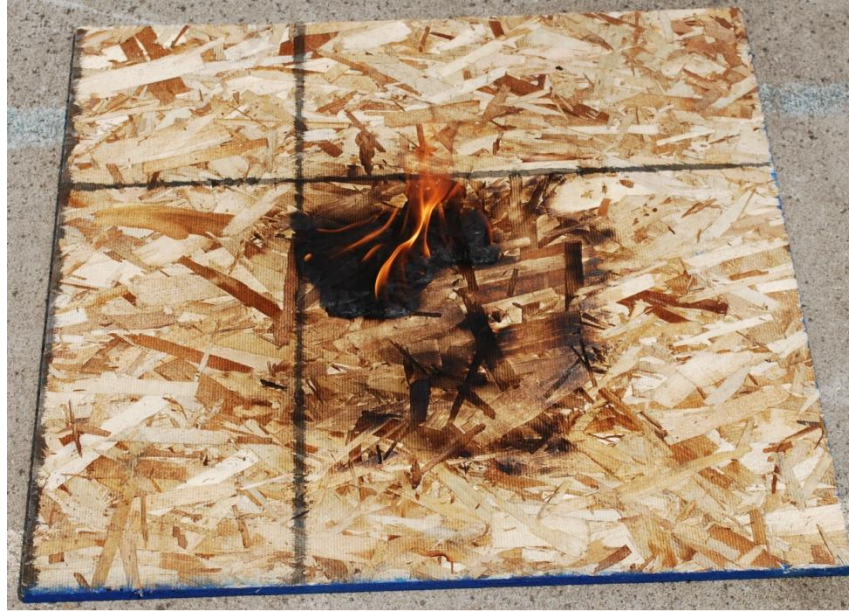
Figure 35: Burn pattern for OSB (50 ml of kerosene)
