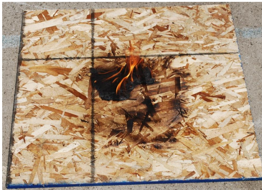
Figure 35: Burn pattern for OSB (50 ml of kerosene)
