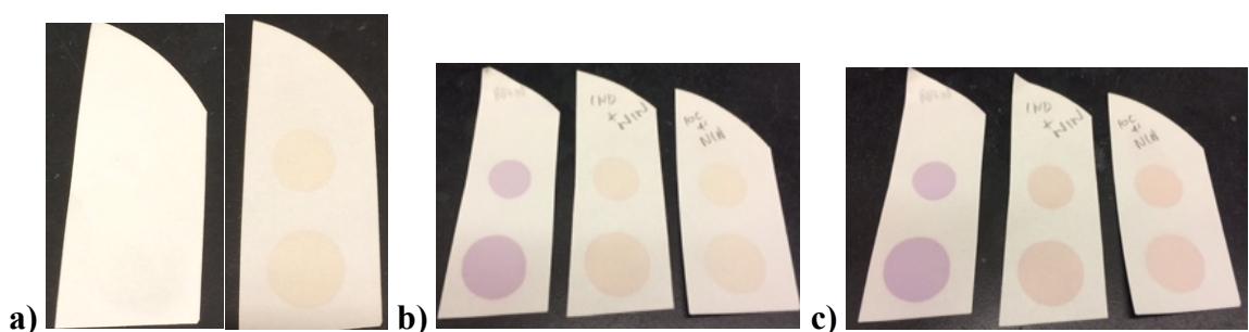
Figure 5.4. Spot test results; a) Initial treatment with 53 (left), post treatment with ninhydrin (right) b) Ninhydrin (left), 1,2-indanedione with ninhydrin post treatment (middle), 53 with ninhydrin post treatment (right) c) After 24 h.
