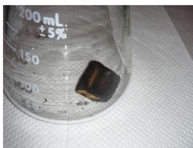
**Figure 3-26.** Post-burn wood block visibly charred and cracked after ignition with Coleman Fuel. Generated headspace can then be analyzed directly via APCI-MS
