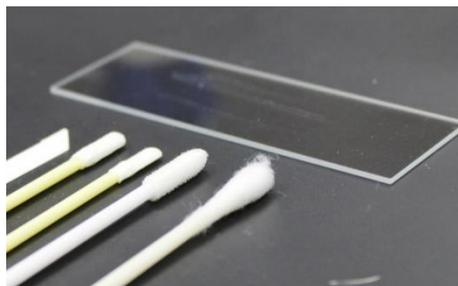
**Figure 3-18.** Examined commercial swabs. From left to right: Whatman chromatography paper used for PSI-MS, woven fiber, non-woven foam, polyurethane foam buccal, and spun cotton “Q-Tip”-style. Also seen is a residue-containing glass slide used for physical transfer studies.
