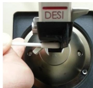
**Figure 3-21.** Photo of DESI swab analysis utilizing a swab positioning guide from Flir Mass Spectrometry.
