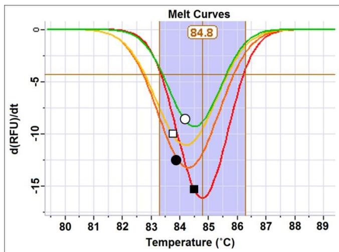
Figure 5: Melt curve effects of bile salts on 53% GC 160bp at concentrations of 0 (red ■), 0.5 (orange ●), 1.0 (yellow □) and 1.5ng/μL (green ○) indicating an initial decrease in  $T_m$  followed by a gradual increase in  $T_m$  as inhibitor concentration increases. From this, it is possible that the melt may not give any indication to the presence of bile salts if the concentration is sufficiently high.
