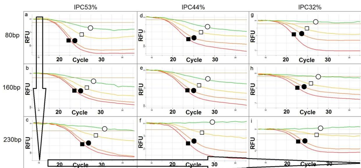
Figure 3: Combined effects of amplicon size (increasing downward) and GC content (decreasing left to right) sequence in urea at concentrations of 0 (red ■), 100 (orange ●), 300 (yellow □) and 500mM (green ○) indicating that as the amplicon size increases and as the sequence %GC content decreases, the DNA's sensitivity to inhibition can increase. Arrows indicate increasing size and decreasing GC content.
