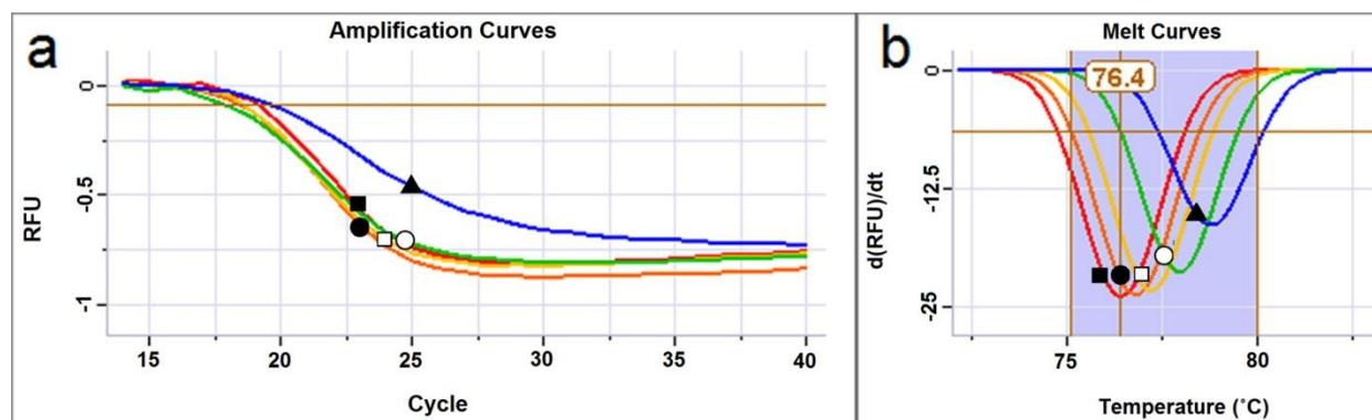
Figure 4: Amplification and melt curves of 44% GC and 80bp amplicon with 0 (red ■), 25 (orange ●), 50 (yellow □), 75 (green ○) and 100ng/μL (blue ▲) of collagen. With the IPCs, increasing concentrations of collagen show little change from the control while the melt curves shift greatly with increasing inhibitor concentration.
