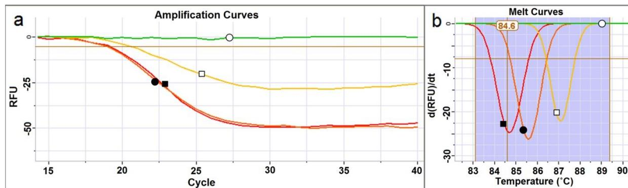
Figure 3: Amplification and melt curves of IPC 53% 160bp amplicon with guanidinium concentrations at 0 (red ■), 1.5 (orange ●), 4.5 (yellow □) and 7.5ng/μL (green ○). This set of amplification curves shows how at low amount of inhibition, it is possible to not detect it during the amplification phase (a), but using melt curves, it is possible to differentiate between an inhibited and uninhibited sample (b).
