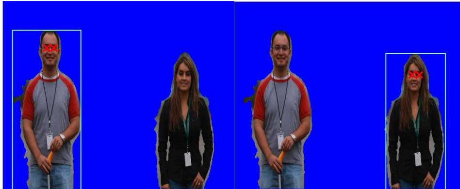
**FIG. 15: Example of automatic eye localization of auto-segmented objects. These segmented objects are then “fed” one at a time into the 2D engine and compared against a 2D database of faces for identification.**
