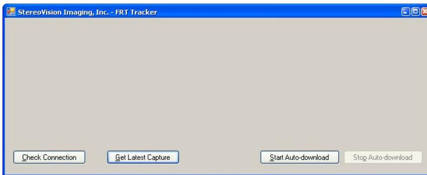
Once the FRT 3DVuCAM™ is powered and connected to the laptop, you may click on the **Check Connection** button to ensure that communication to the FRT 3DVuCAM™ from the laptop is unhindered. You should see the following notification:
