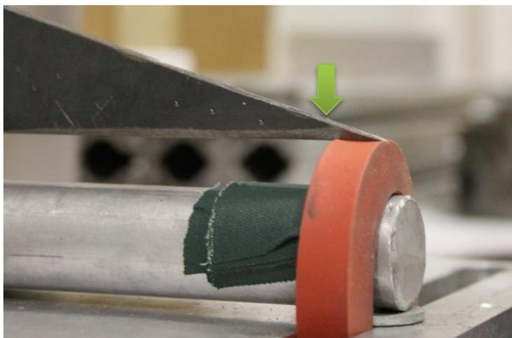
**Figure 16:** Edge sharpness test setup.
