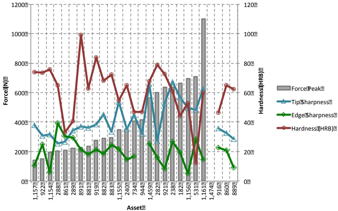
Figure 23: Push-through blade test performance and attributes.
