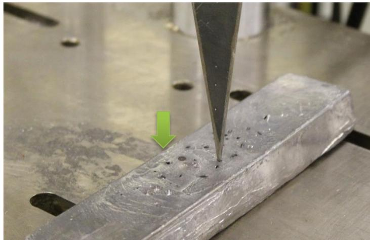
**Figure 14:** Tip sharpness indenter test setup.
