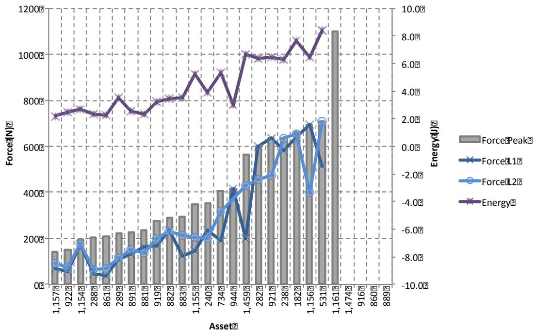
Figure 21: Push-through bladed weapon force test results.
