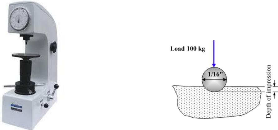
**Figure 17:** A typical Rockwell Hardness tester and Rockwell "B" spherical ball indenter.
