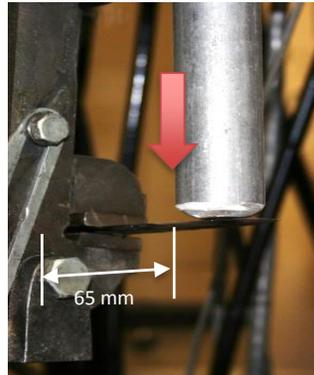
**Figure 28:** Experimental setup for flexural stiffness (courtesy of WSU).
