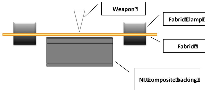
**Figure 18:** Push-through test components and setup
