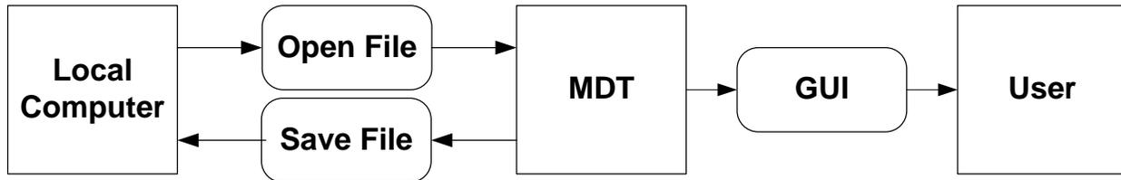
**Figure 1: MDT External Interface Diagram**
