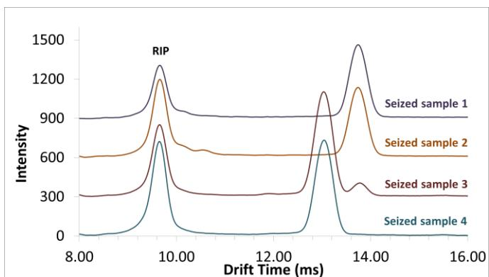
Figure 3. Overlaid ion mobility spectra of four seized samples analyzed by the Barringer IMS.
