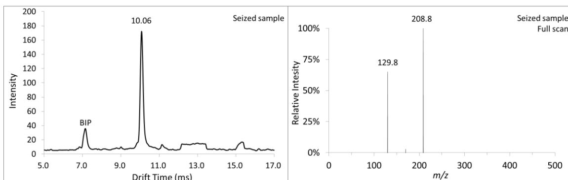
Figure 4. Ion mobility spectrum (left) and corresponding mass spectrum (right) of the seized drug sample by the Excellims ESI-IMS-MS.
