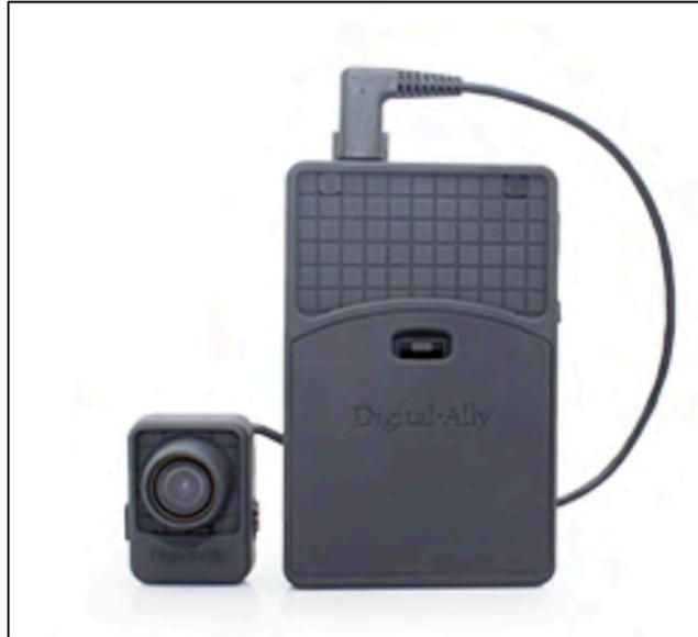
**Figure 11. Digital Ally FirstVu HD Body Worn Camera**
