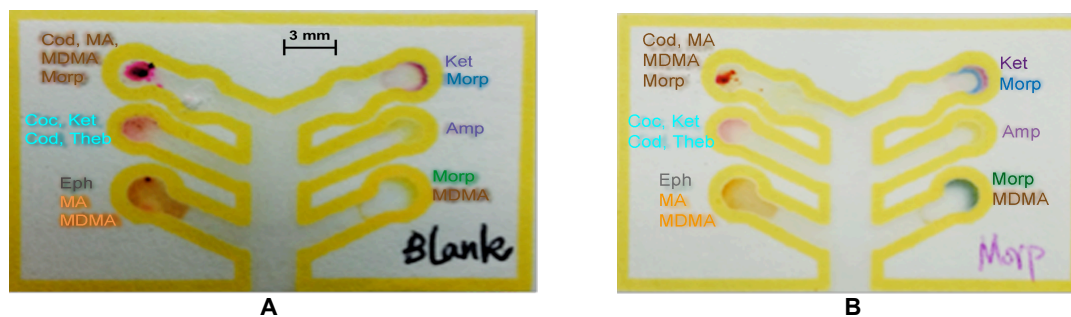
Figure 6. A demonstration of our microfluidic paper-based device for the detection of seized drugs in a blank sample ( A ) and a sample adulterated with morphine (Morp) ( B ). Each lane is labeled with the name of analytes and the color they should produce. Lane 1, ephedrine (Eph), metamphetamine (MA) and MDMA; Lane 2, cocaine (Coc), codeine (Cod), ketamine (Ket) and thebaine (Theb); Lane 3, Cod, MA, MDMA and Morp; Lane 4, Ket and Morp; Lane 5, amphetamine (Amp); Lane 6, Morp and MDMA.
