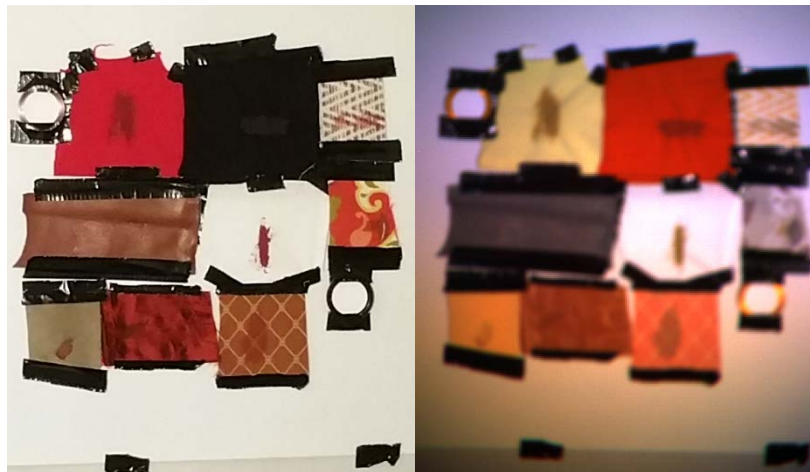
Figure 1: (a) A set of targets including leather (far left of middle row) and various patterned cloth upholstery stained with pig blood. The white disks in the image are used to calibrate the spectral content of the illumination source. Image acquired with a cell phone camera. (b) False color RGB image which retains the Blue (420 nm) and Green (500 nm) channels but replaces the Red channel with IR spectral data at 780nm. The contrast in the blood stains relative to the black shirt and patterned materials improves relative to 'normal' RGB images.
