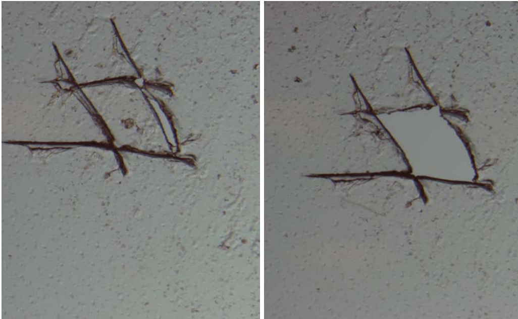
Figure 4: Fingerprint on SIRCHIE tape: Skin flake is visible (right panel), the tape was cut using an X-Acto knife (right panel) and removed (left) using Dumont tweezers (observed under Axiozoom, 20x magnification).
