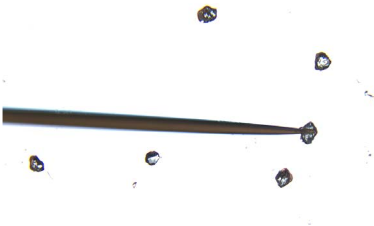
Figure 2: Arabic gum/glycerol spheres (approximately 200 \mu\text{m} in diameter, 80x magnification, Axiozoom) can be used to lift single cells. One sphere is held with the tip of the tungsten needle (Axiozoom).
