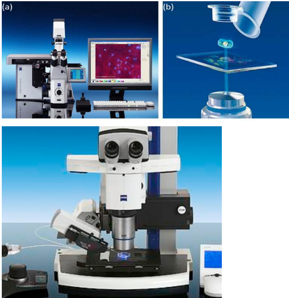
Figure 16: Top: PALM system and laser ablation of a membrane slide on inverted microscope (pictures taken from (61)). Bottom: Axiozoom and aureka® micromanipulator (36).
