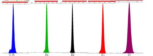
**Figure 23:** CE results of a single amplicon from each colored nuorophore. Markers 4 (blue), 2 (green), 5 (yellow), 8 (red), and 20 (purple).
