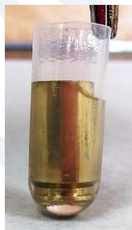
Figure 1. Example of pipette bulb as the soaking vessel for a casing in 700uL of digestion/tissue lysis buffer.
