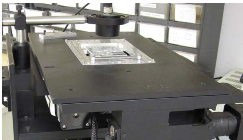
**Figure 10** The microfluidic substage mounted on the XY translation stage. The valve manifold is out of sight, underneath the translation stage.
