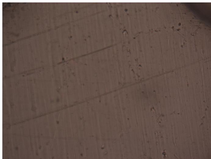
**Figure 6** Surface imperfections in a molded COC microfluidic channel, viewed with bright-field microscopy.
